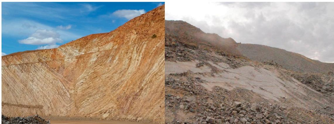
**Figure 4.** (Left): near-laminated weathered siltstone with siltstone-siltstone bedding planes (Telfer Gold mine, Australia). (Right): planar failure in fresh quartzite with quartzite-quartzite bedding planes (Telfer Gold Mine, Australia). Both have bedding scale anisotropy [28].
