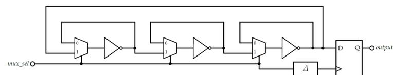
Figure 2. Metastable Ring Oscillator.
