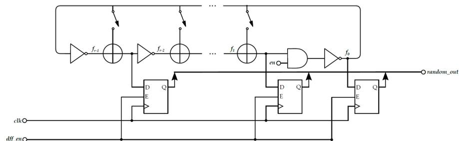
Figure 12. Galois Ring Oscillator with state sampling. The output bus is XORed together to form a 1-bit output in the higher level.
