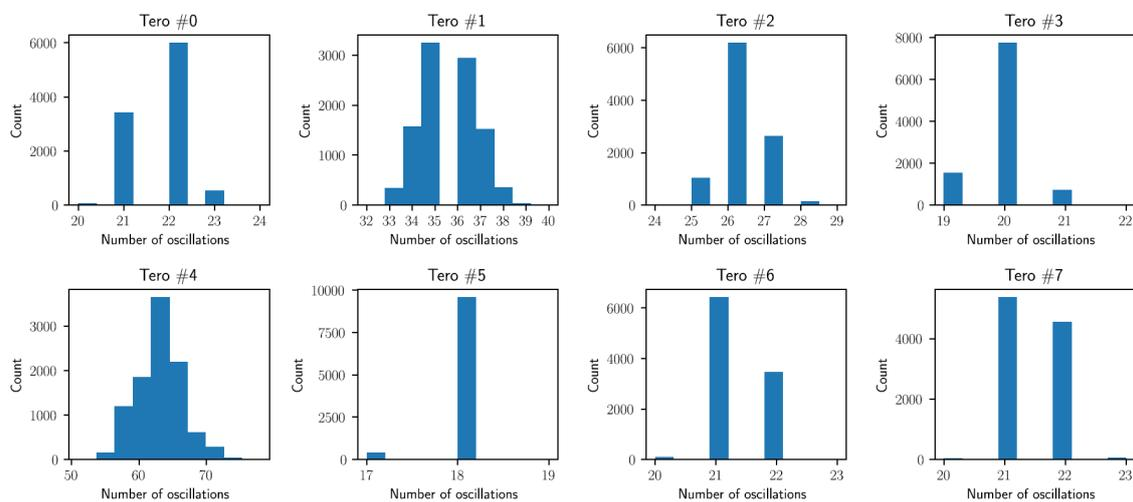
**Figure 8.** Number of oscillations histogram for  $10^5$  trigger events for Transition Effect Ring Oscillator (TERO) True-Random Number Generator (TRNG).
