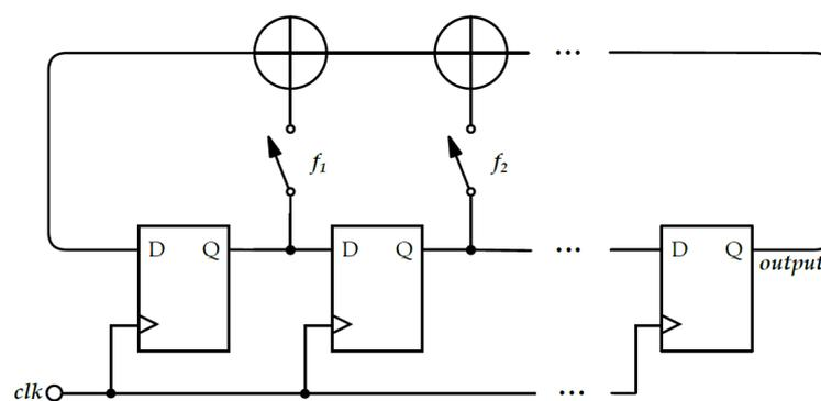
Figure 3. Fibonacci Linear Feedback Shift Registers.
