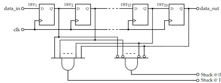
**Figure 14.** Hardware implementation of the repetition count test for a binary random source.
