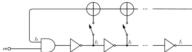
Figure 5. Fibonacci Ring Oscillator with enable port.
