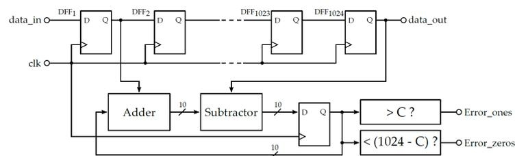
**Figure 15.** Hardware implementation of the adaptive proportion test for a binary random source.
