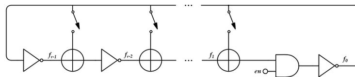
Figure 6. Galois ring oscillator with enable port.
