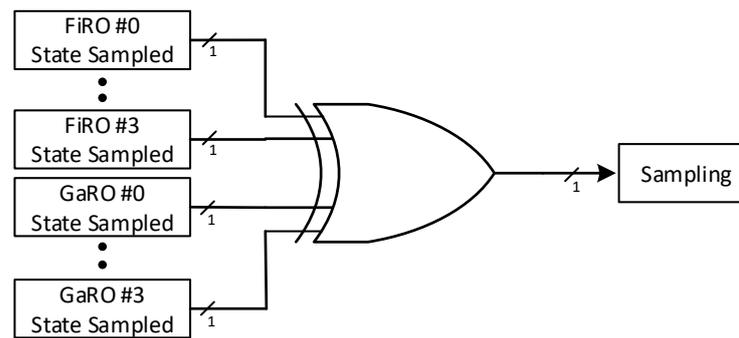
**Figure 7.** Fibonacci-Galois Ring Oscillator (FiGaRO) four elements architecture.
