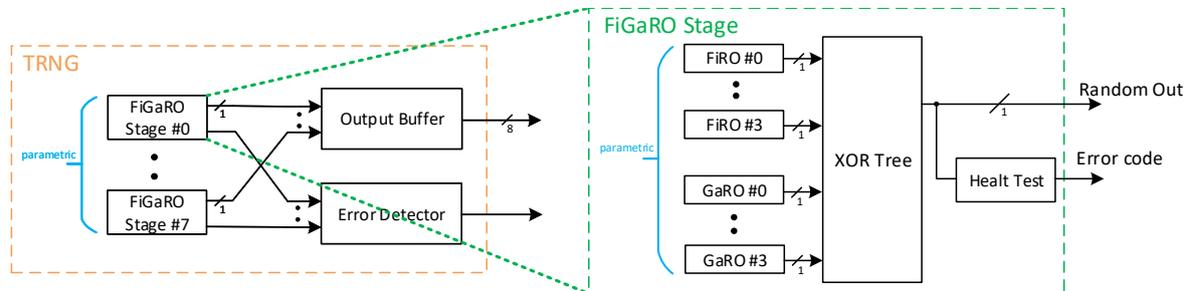
Figure 16. Overall architecture of the implemented FiGaRO Random Number Generator (RNG).
