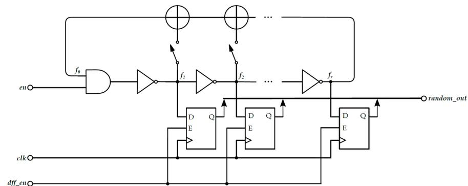
Figure 11. Fibonacci Ring Oscillator with state sampling. The output bus is XORed together to form a 1-bit output in the higher level.
