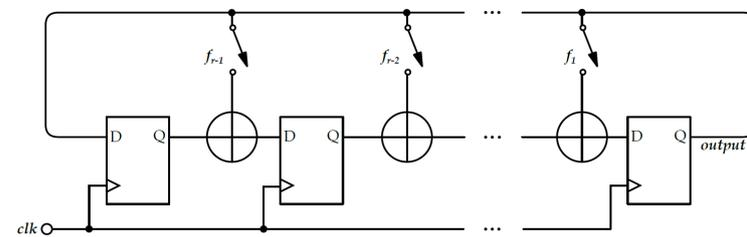
Figure 4. Galois Linear Feedback Shift Register.
