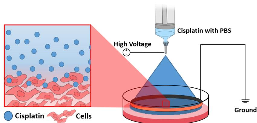
**Figure 1.** Schematic diagram of the cisplatin delivery-based electrospray (CDES) system. The CDES system facilitated the delivery of cisplatin to cancer cells. This method suggested a way to kill cancer cells by treating drugs locally into the tumor tissue.
