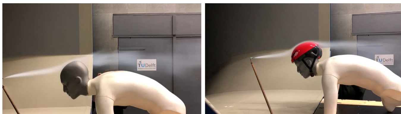
Figure 14. Smoke flow visualization on the head of the skater mannequin for the bare head case (left) and the Omega helmet case (right).
