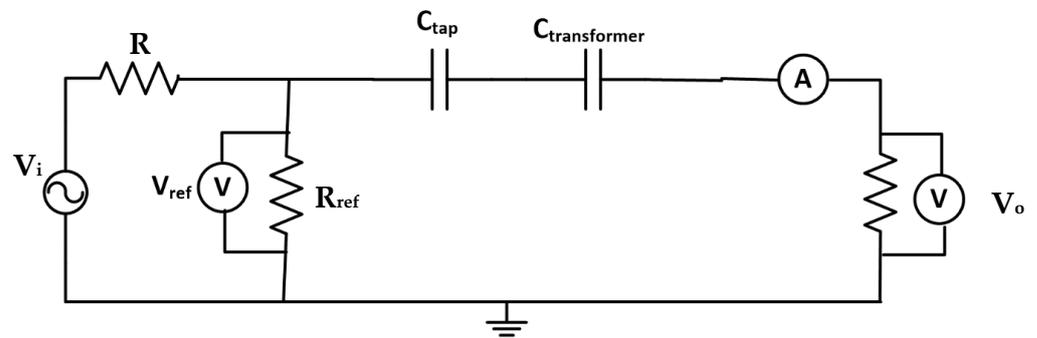
Figure 16. Capacitive interwinding test configuration.
