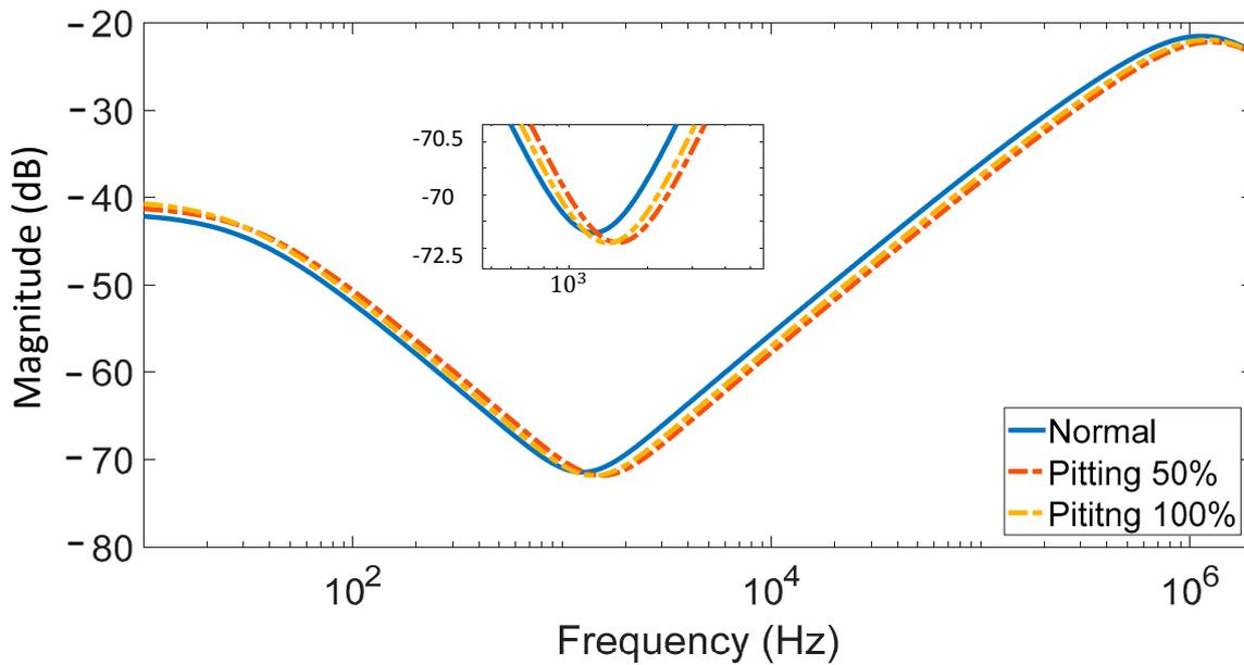
Figure 11. Simulated FRA for normal, vs. 50% pitting and 100% pitting.
