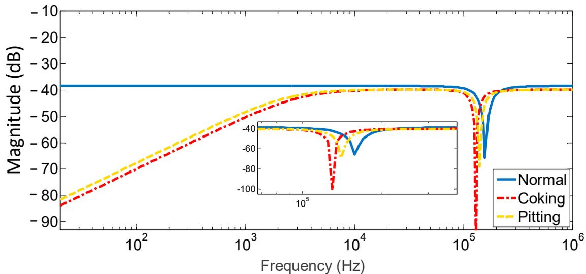
**Figure 20.** Simulated FRA for normal, vs. 100% coking and 100% pitting.
