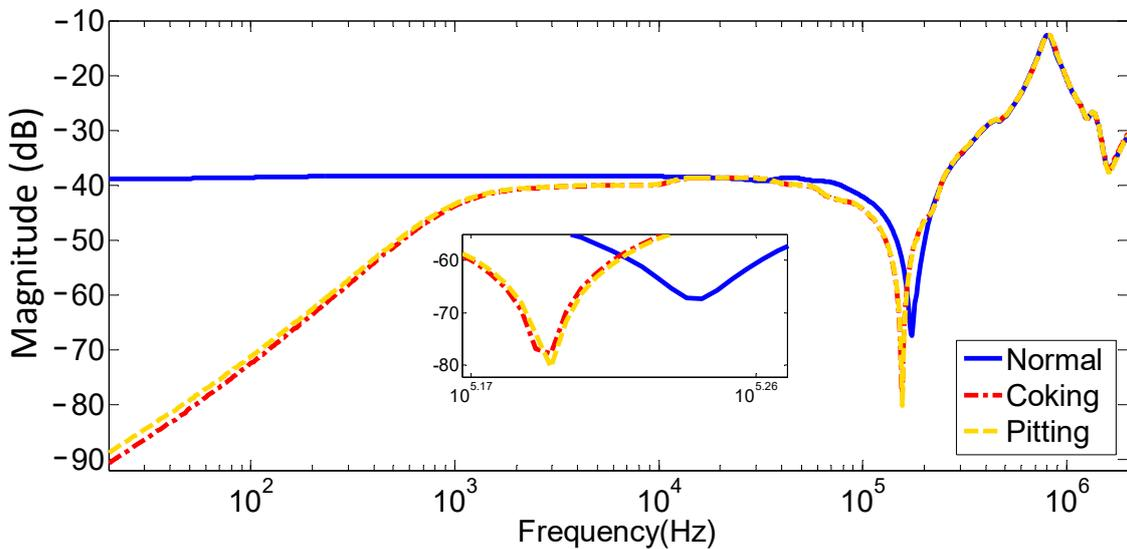
**Figure 19.** Measured FRA for normal, 100% coking, and 100% pitting.
