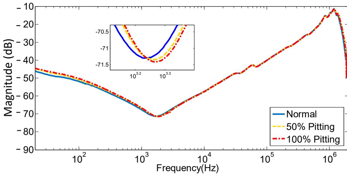
Figure 10. Measured FRA for normal, vs. 50% and 100% pitting.
