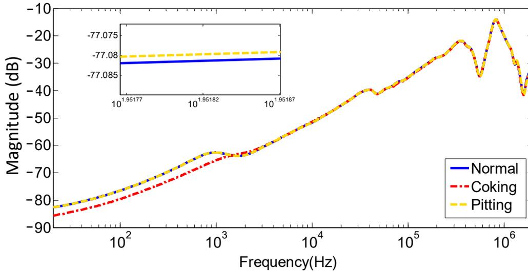
Figure 15. Measured capacitive interwinding FRA for normal vs. 100% coking and 100% pitting tap conditions.
