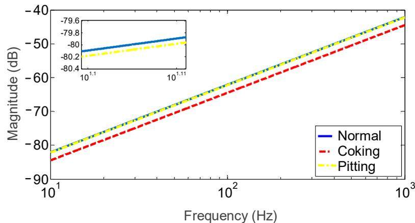
Figure 17. Simulated capacitive interwinding FRA for normal vs. 100% coking and 100% pitting tap conditions.
