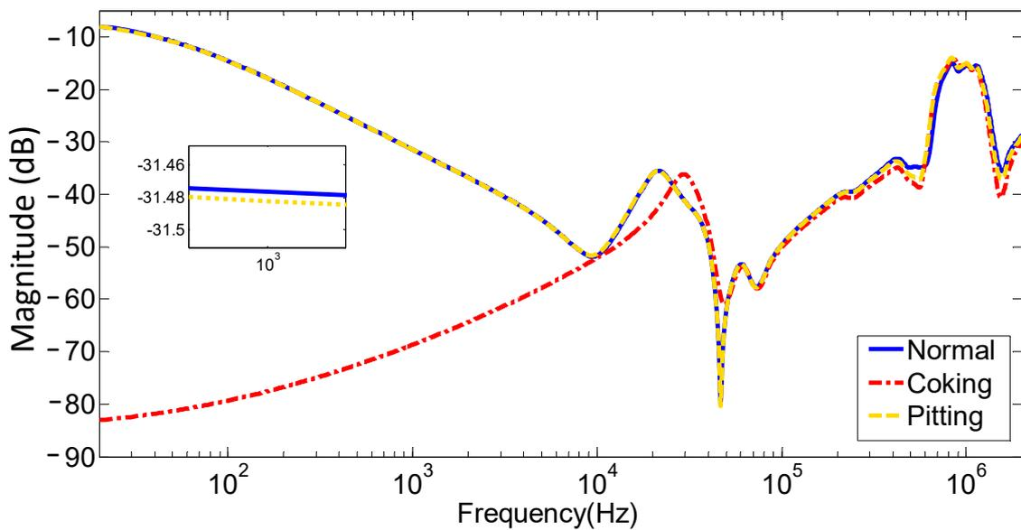
Figure 13. Measured FRA for normal, vs. 100% coking and 100% pitting.
