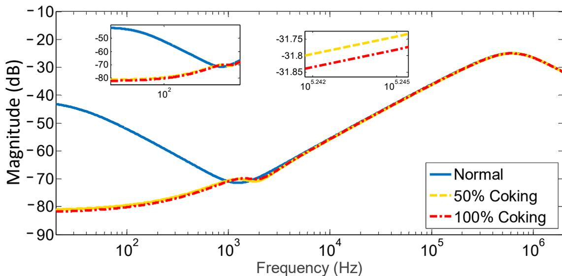
Figure 9. Simulated FRA for normal, vs. 50% and 100% coking.
