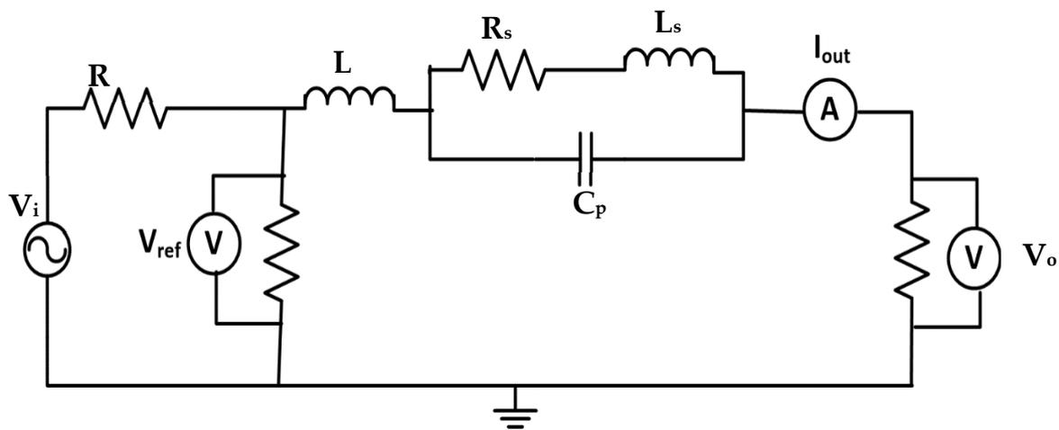
Figure 6. Simulated tap changer RLC circuit using MATLAB/Simulink.
