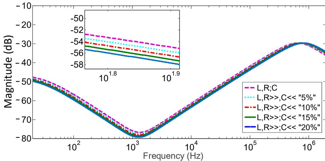
Figure 7. Simulated FRA for all tap changer positions.
