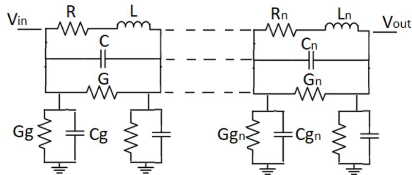
Figure 5. Equivalent schematic resistance, inductance, and capacitance RLC network of transformer winding.
