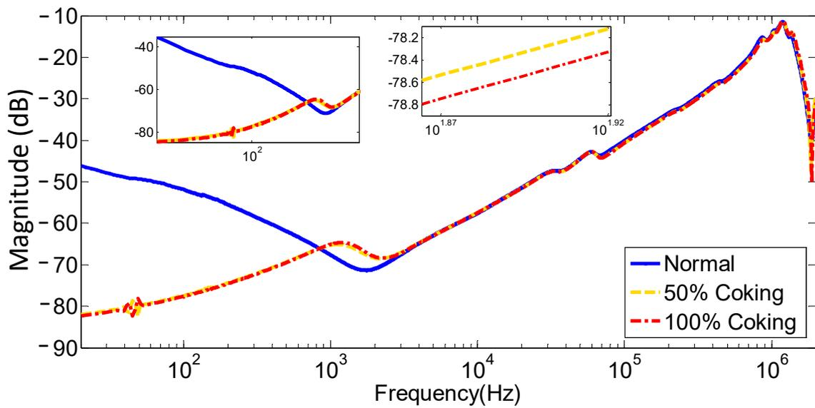
Figure 8. Measured FRA for normal, 50%, and 100% coking.
