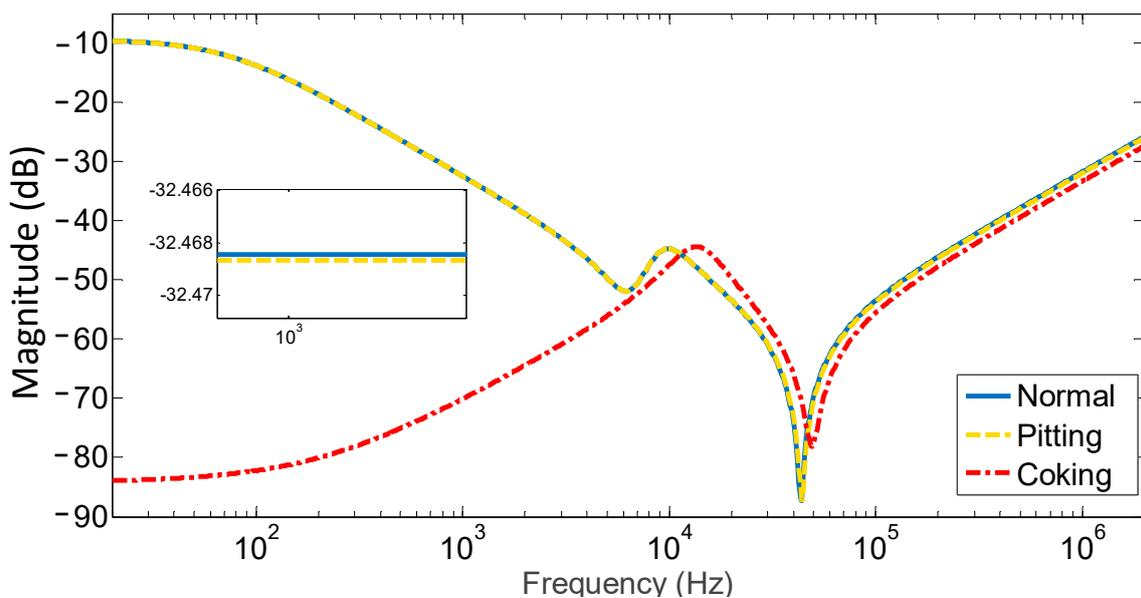
Figure 14. Simulated FRA for normal, vs. 100% coking and 100% pitting.
