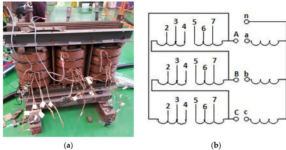
**Figure 1.** (a) The 11/0.415 kV, 500 kVA distribution transformer and (b) winding configuration.
