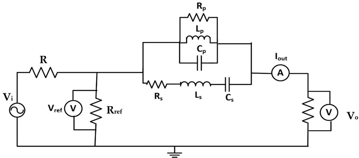
Figure 12. The RLC circuit model for the tap changer under the FRA short circuit test.
