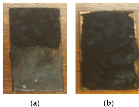
**Figure 2.** Tap contacts coking (a) 50% and (b) 100%.
