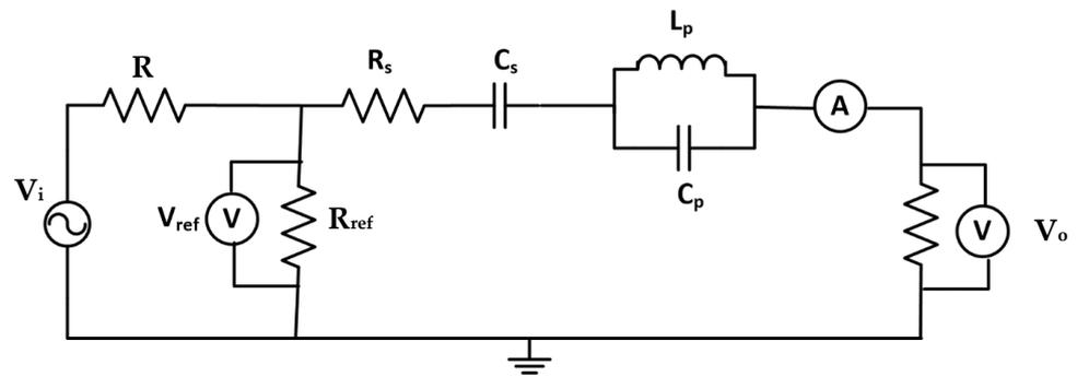
**Figure 18.** Inductive interwinding test configuration.
