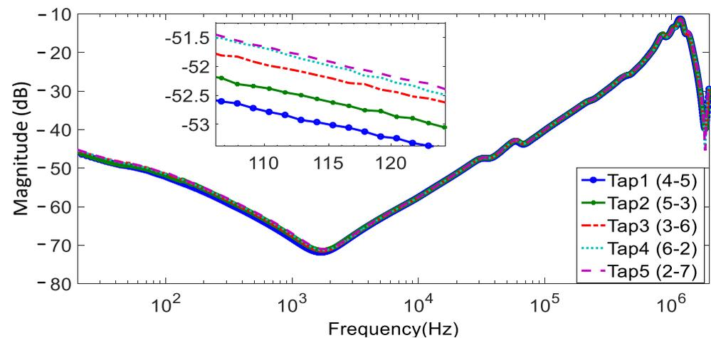
Figure 4. Measured frequency response analysis (FRA) at all tap changer positions.
