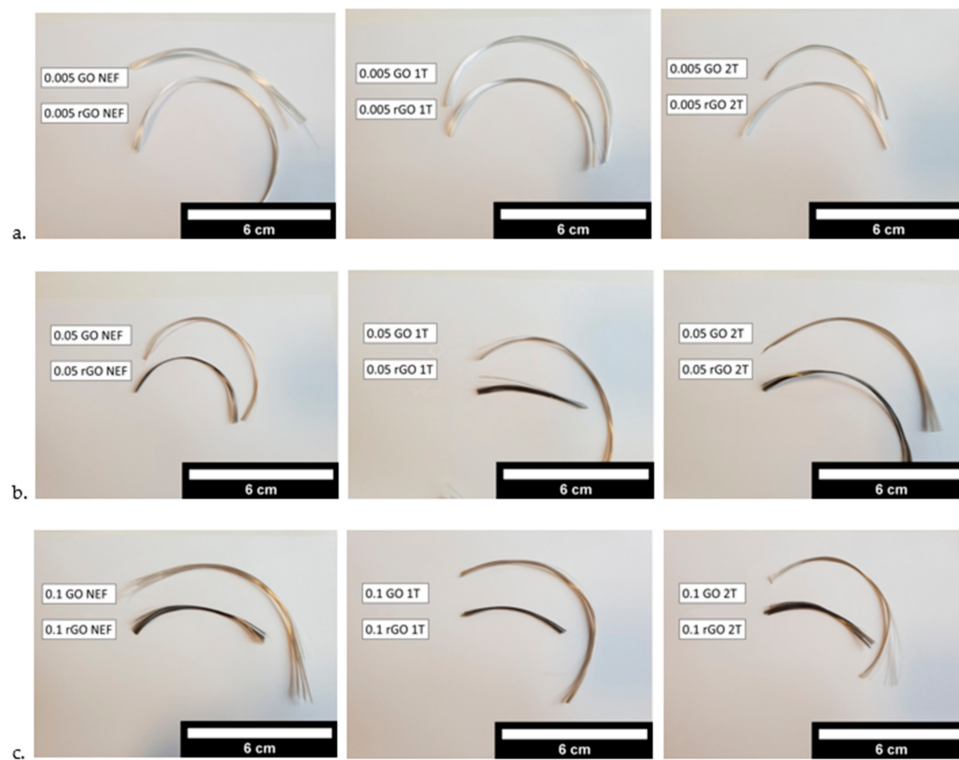
Figure 3. Representative images of (a) 0.005 GO/rGO, (b) 0.05 GO/rGO, (c) 0.1 GO/rGO fibers (NEF, 1T, 2T).
