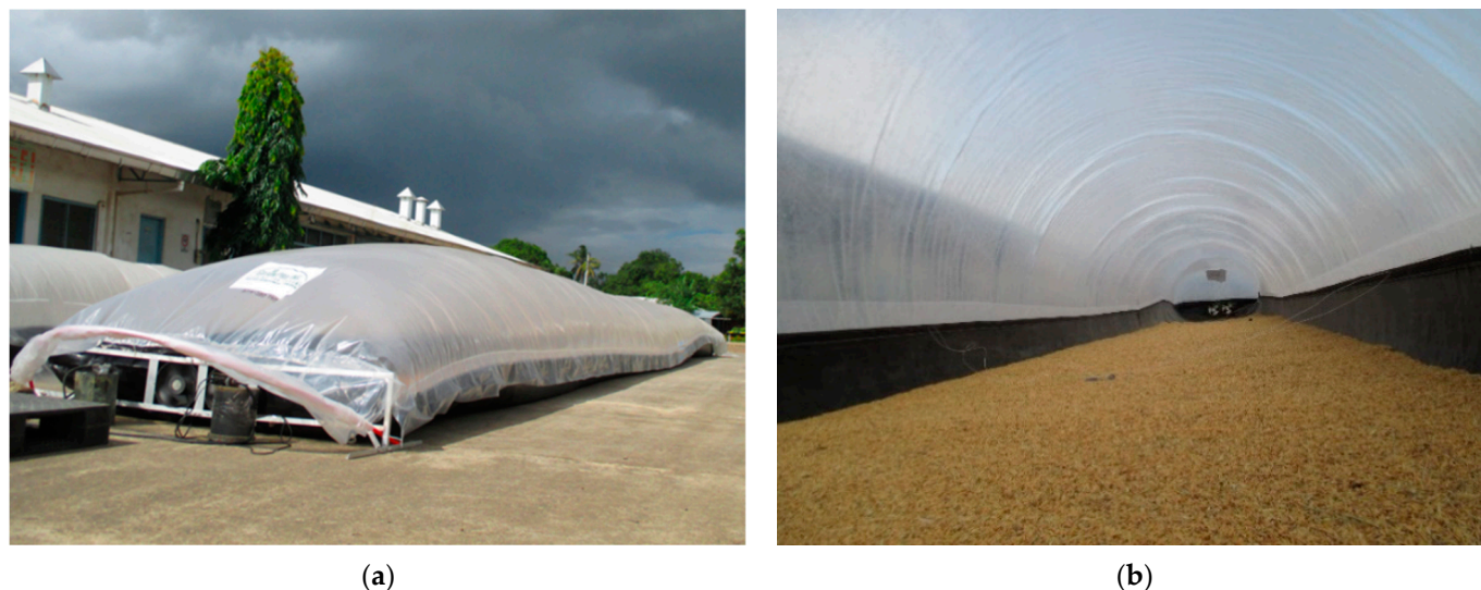
Figure 1. Inflatable solar dryer: (a) perspective view and (b) inside of the dryer.
