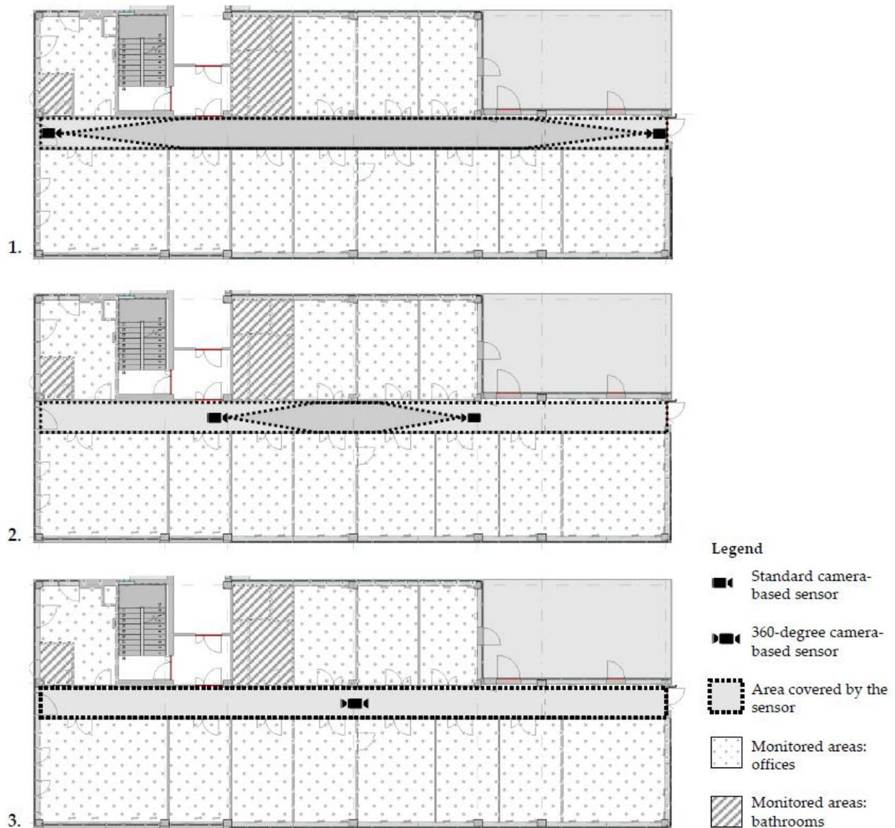
**Figure 4.** 2D visualization of the three simulations of sensors positioning in a typical corridor through the BIM model.
