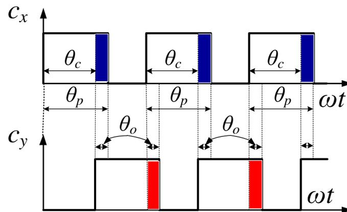
**Figure 4.** Inductor current elimination through turn-off delay angle.
