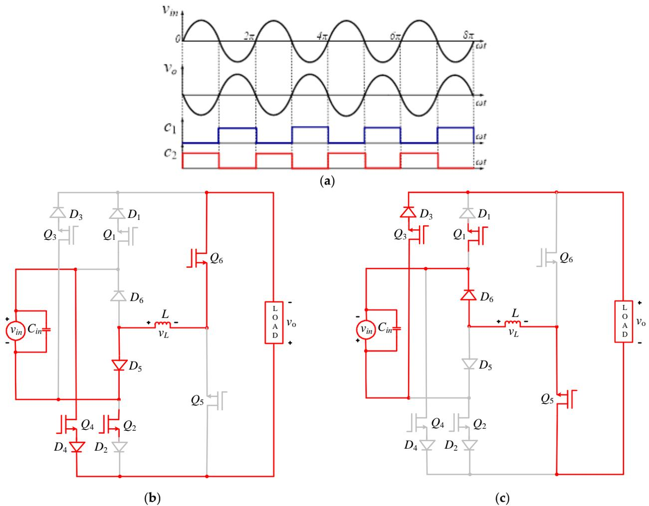
**Figure 6.** Voltage inverting operation: (a) switching control scheme; (b) current closed-loop during positive input; (c) current closed-loop during negative input.
