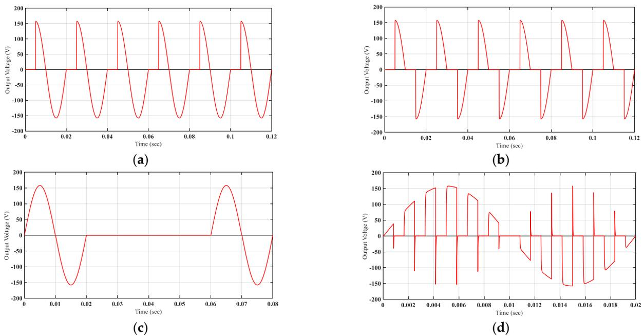
**Figure 14.** Output voltage control through (a) phase angle half-wave control; (b) phase angle full-wave control; (c) number of on-off cycles control; (d) PWM control.
