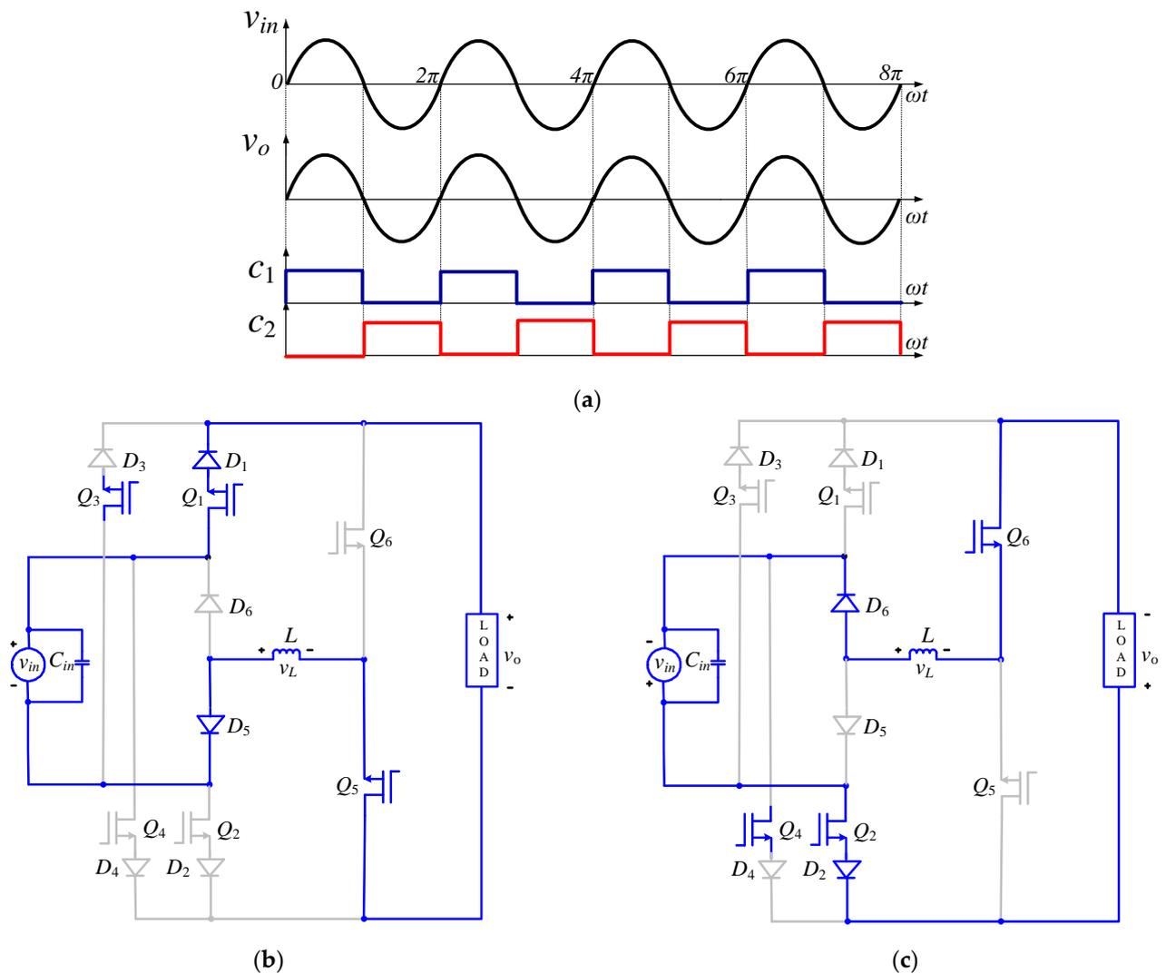
**Figure 5.** Voltage non-inverting operation: (a) switching control scheme; (b) current closed-loop during positive input; (c) current closed-loop during negative input.
