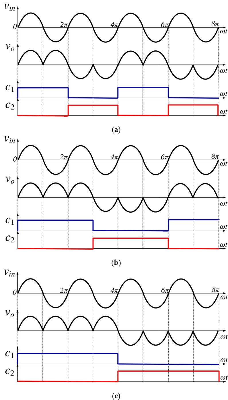
**Figure 9.** Output step down frequency control with respect to input frequency: (a) one-half; (b) one-third; (c) one-fourth.
