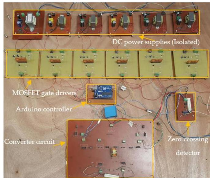
**Figure 15.** The practical architecture of the proposed converter.
