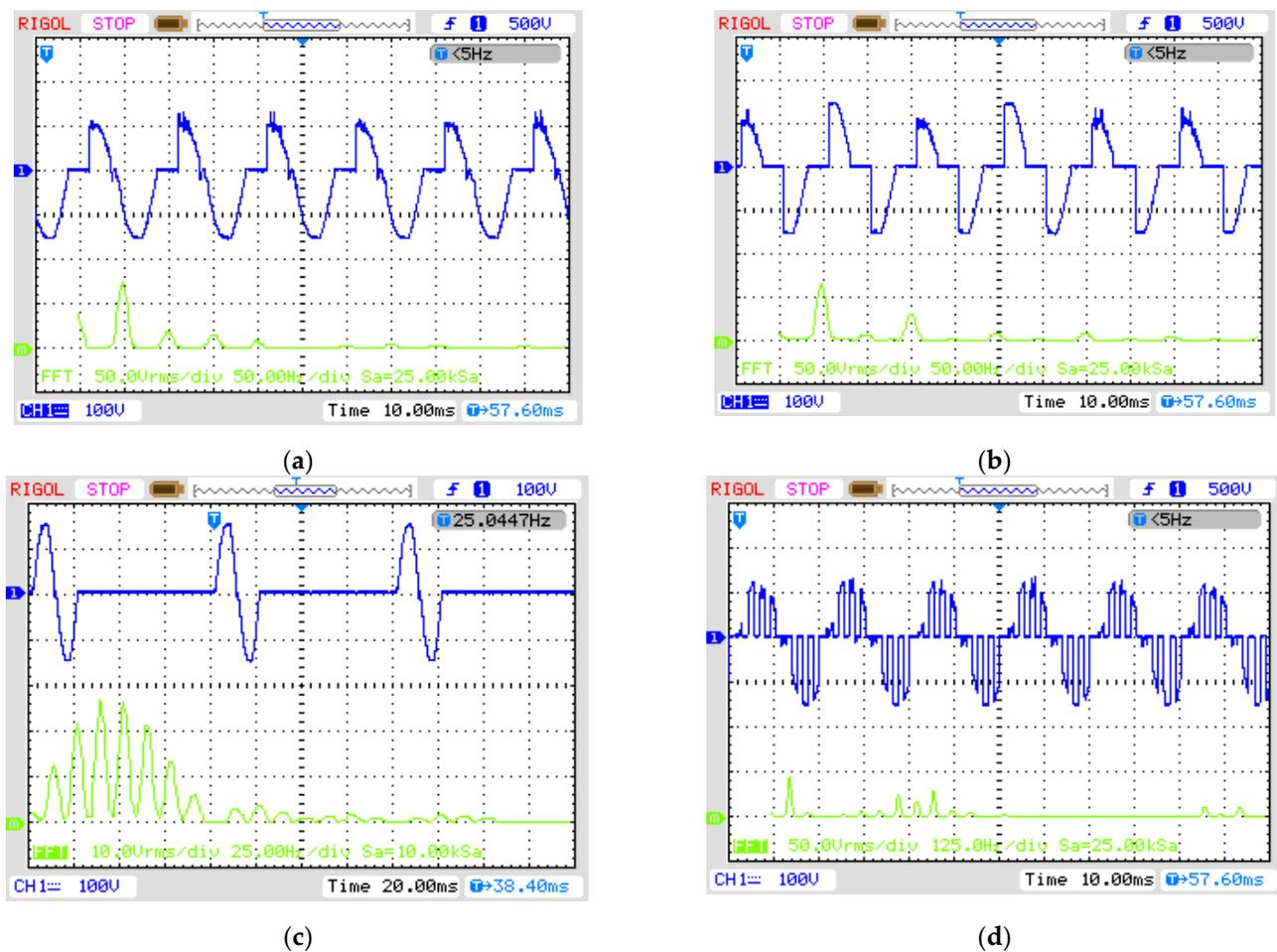
**Figure 20.** RMS voltage control at the output through (a) phase angle half-wave control; (b) phase angle full-wave control; (c) a number of on-off cycles control; (d) PWM control.
