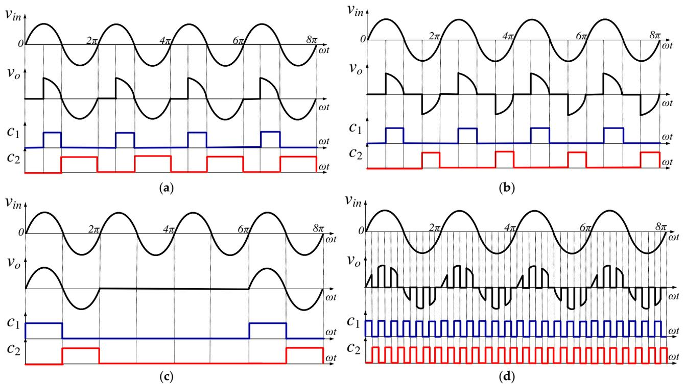
**Figure 8.** Output rms voltage control: (a) half-wave control; (b) full-wave control; (c) on-off cycle control; (d) PWM chopping.
