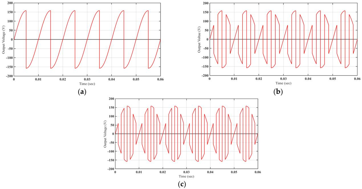
**Figure 13.** High frequency outputs with respect to constant input frequency (50 Hz): (a) 2(50) Hz; (b) 3(50) Hz; (c) 4(50) Hz.
