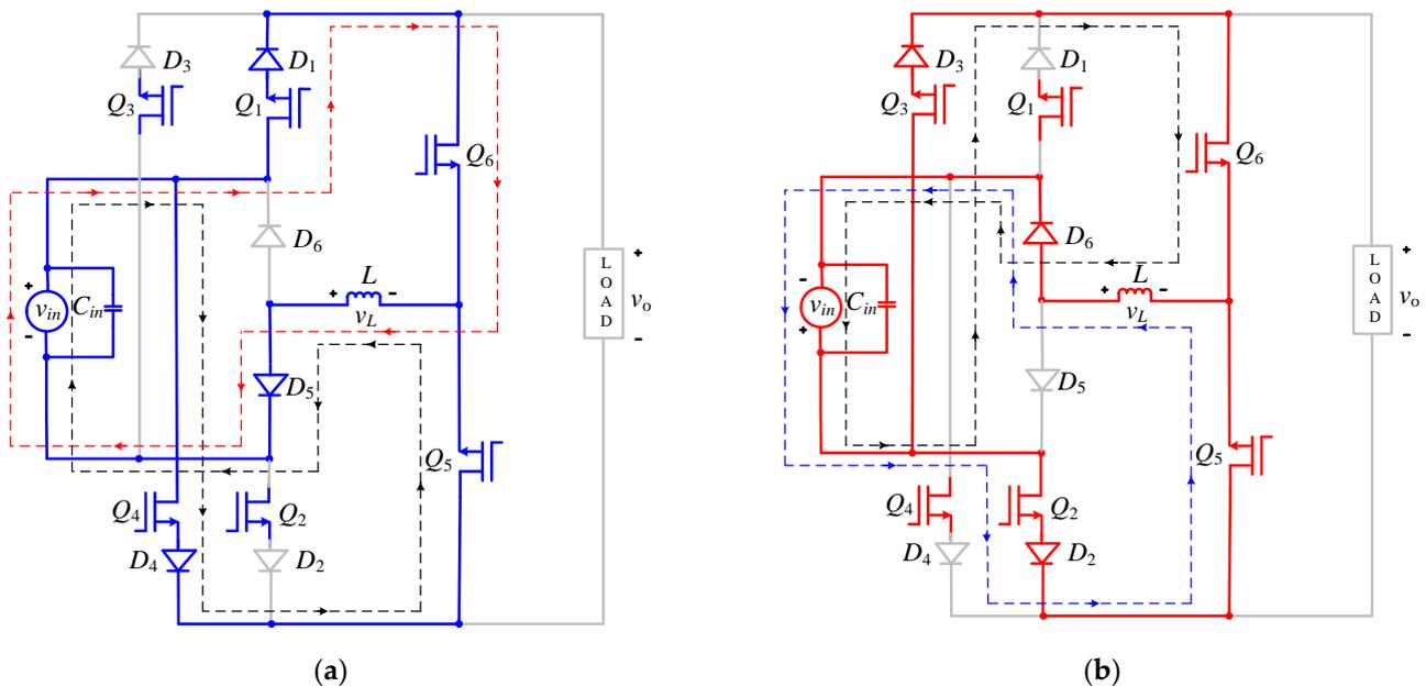
Figure 3. Currents loops during shoot-through operation for (a) positive input and (b) negative input.
