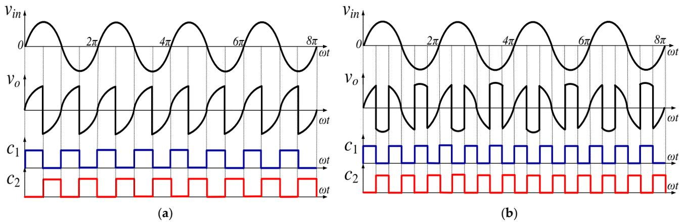
Figure 10. Output step-up frequency control with respect to input frequency: (a) two times; (b) three times.
