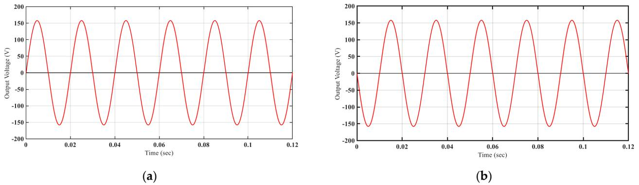
**Figure 11.** Constant frequency (50 Hz) outputs during: (a) non-inverting state; (b) inverting state.
