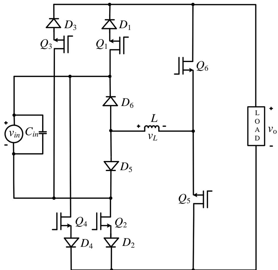
**Figure 2.** Schematic view of the suggested topology.
