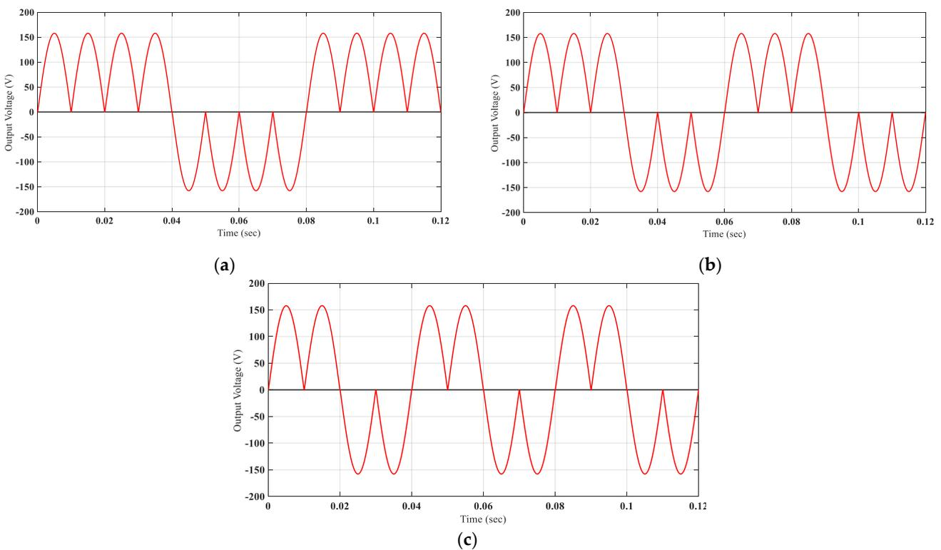
**Figure 12.** Low-frequency outputs with respect to constant input frequency (50 Hz): (a) 50/4 Hz; (b) 50/3 Hz; (c) 50/2 Hz.
