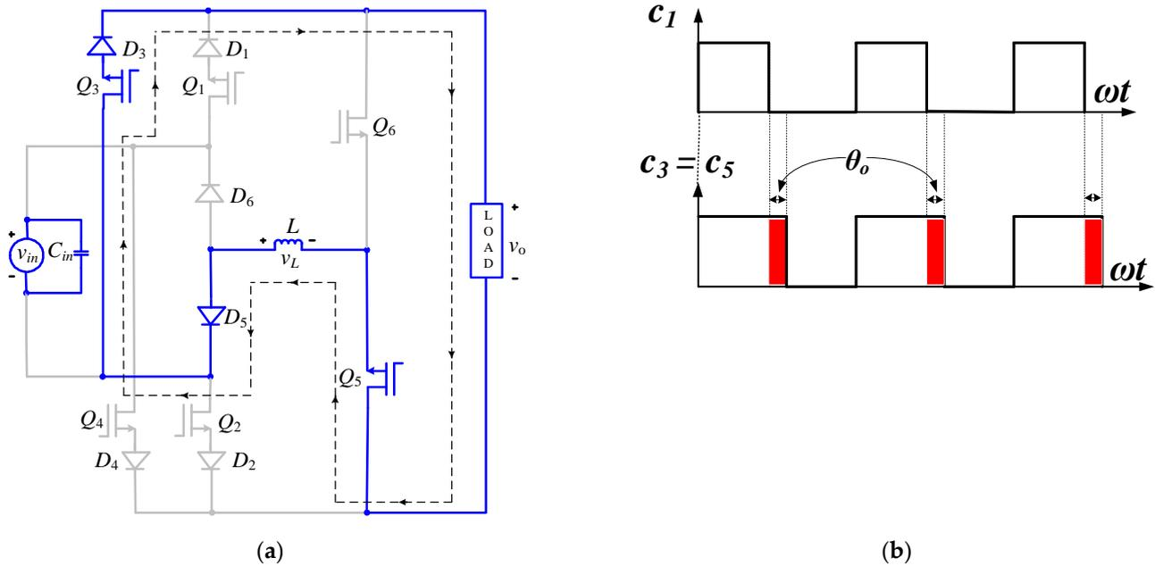
**Figure 7.** Elimination of inductor current interruption during the off state: (a) closed current loop to de-energize the inductor; (b) corresponding switching signals.
