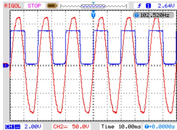
Figure 16. Output of the input voltage sensing circuit.
