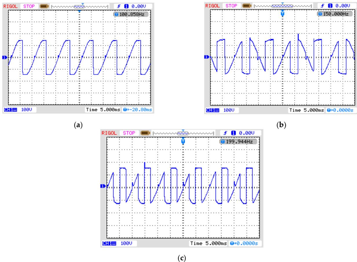
**Figure 19.** Stepping up of standard frequency (50 Hz) at the output to (a) 2(50) Hz; (b) 3(50) Hz; (c) 4(50) Hz.
