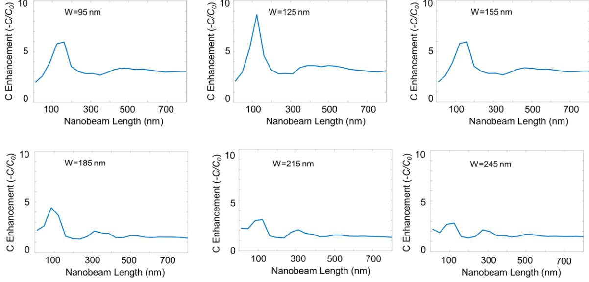
**Figure S2.** C enhancement by changing the length of nanobeam with different widths at the resonance wavelength of 470 nm.
