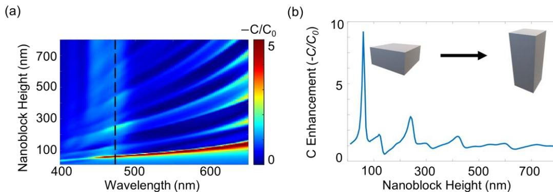
**Figure S1.** (a) Calculated  $C$  enhancement of silicon (Si) nanostructures for the continuously tuned height of the nanostructure. (b)  $C$  enhancement with respect to the heights at the resonance wavelength of 470 nm indicated as the black dotted line in (a).
