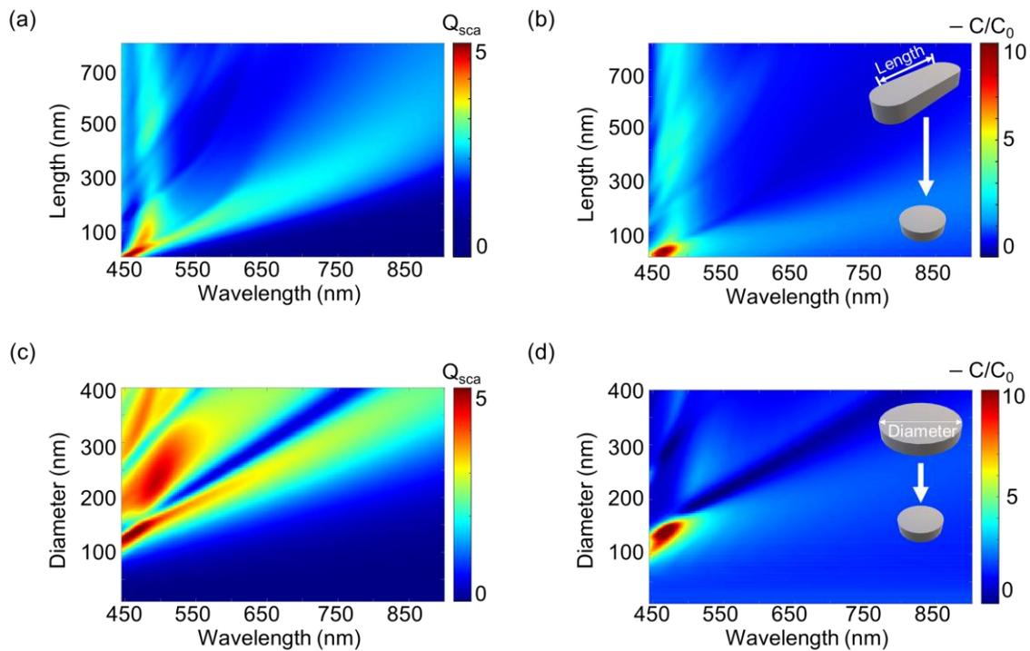
**Figure S4.** (a) Numerically simulated  $Q_{\text{sca}}$  of Si nanostructures for the continuously tuned length of the elliptical nanostructures. (b) Calculated C enhancement of Si nanostructures in (a). (c) Numerically simulated  $Q_{\text{sca}}$  of Si nanostructures for the continuously tune diameter of the circular post nanostructures. (d) Calculated C enhancement of Si nanostructures in (c).
