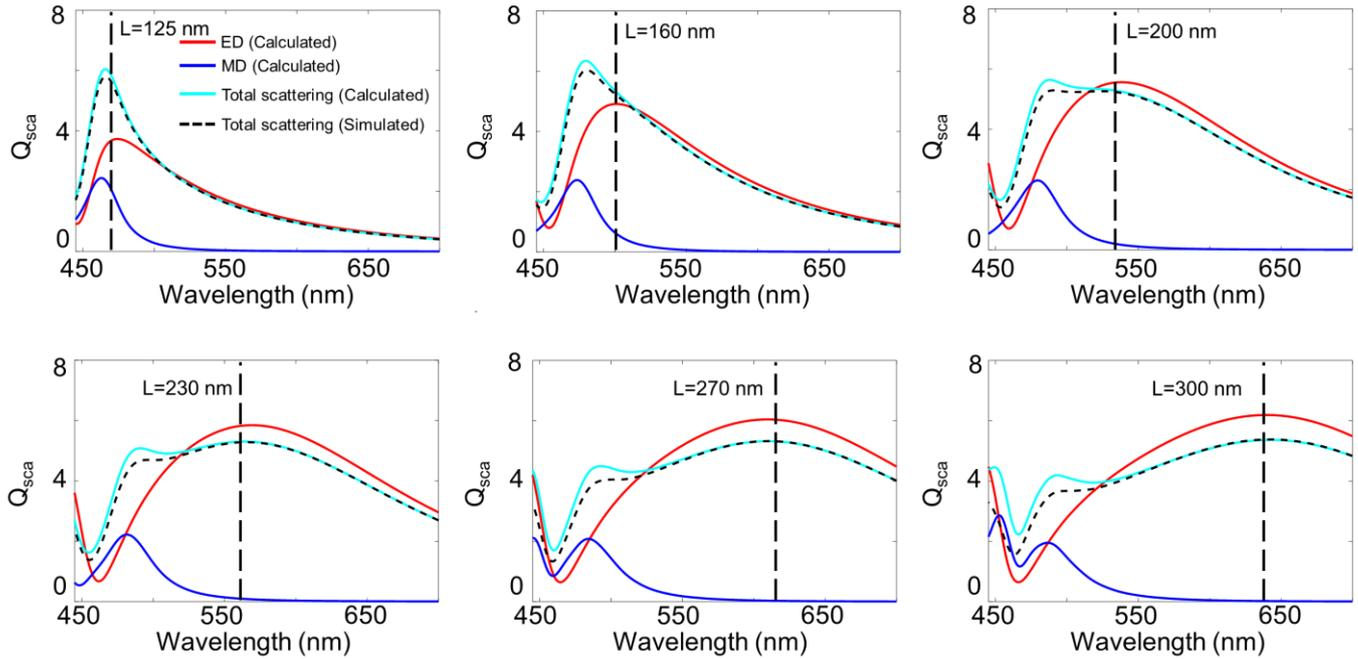
**Figure S3.** Spectrums of theoretically calculated and numerically simulated  $Q_{sca}$  as the length ( $L$ ) of nanobeam is tuned from 95 to 300 nm. Theoretically calculated electric dipole (Red line). Theoretically calculated magnetic dipole (Blue line). Theoretically calculated total scattering (Cyan line). Numerically simulated total scattering (Black dotted line). Vertically black dotted line indicated the ED resonance point.
