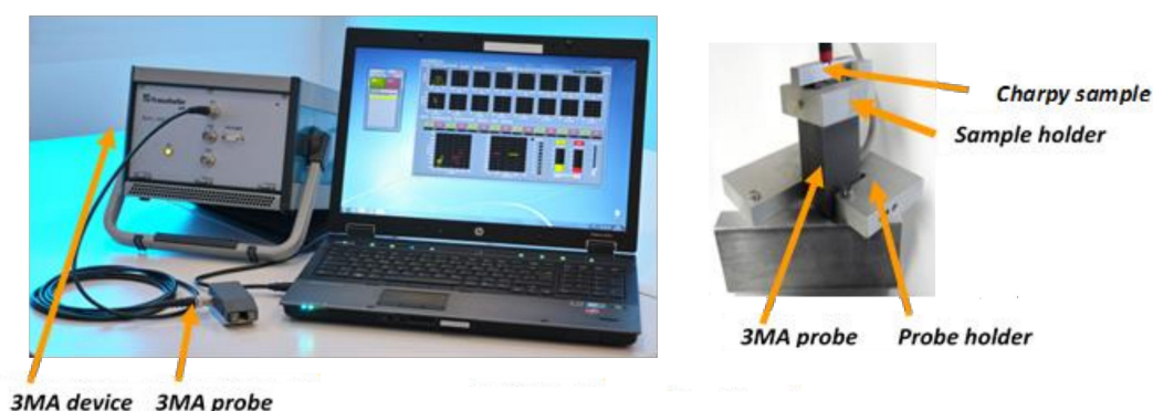
Figure 5. The micromagnetic multiparameter microstructure and stress analysis (3MA)-X8 system, including 3MA-X8 device, probe, and PC (left); (right) specimen holder and probe holder.
