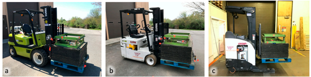
Figure 1. Representative pictures of the investigated forklifts: (a) gas-powered forklift, (b) electric-powered forklift, (c) reach truck.
