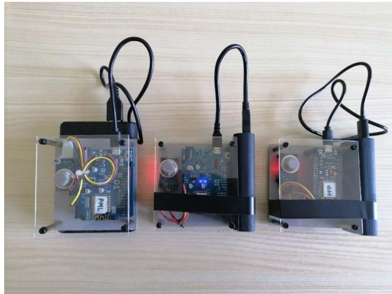
**Figure 6.** Three prototype sensor nodes: two Wemos D1 R2 (left and central), and one NodeMCU (on the right).
