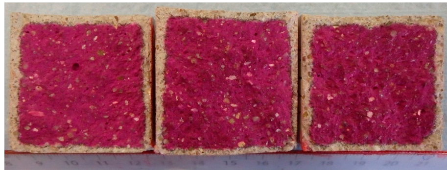
Figure A1. Example of colorimetric carbonation depth assessment after 26 weeks of natural carbonation at 0.04% CO 2 on three fractured surfaces of a CEM II/B-V 42.5 N mortar prism using 1% phenolphthalein color indicator.
