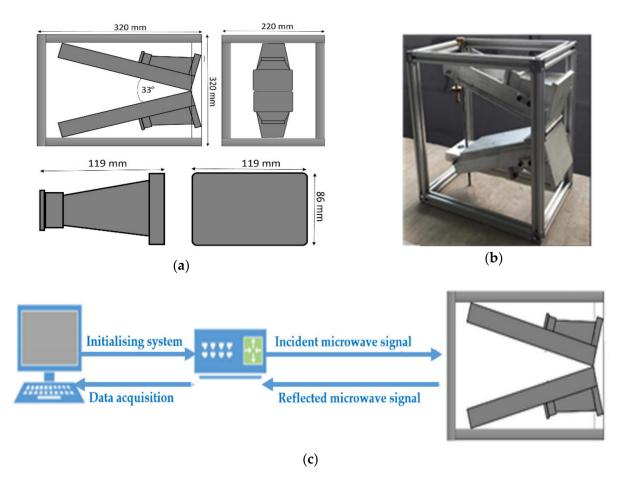
by the LabVIEW GUI in real-time. The dimensions of the bespoke frame with antennas and block diagram of the SFT system is presented in Figure 1.
