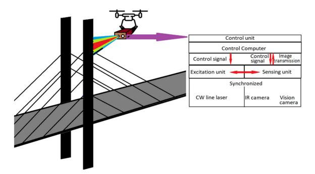
Figure 4. Schematics of the proposed hybrid image scanning (HIS) system [30].
