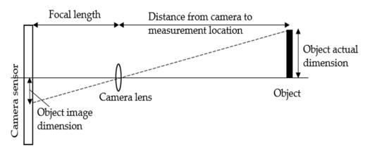
Figure 9. Camera principle [58].
