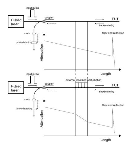
Figure 7. OTDR method-Rayleigh backscattering [32].
