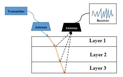
Figure 3. Ground Penetrating Radar principle of work.
