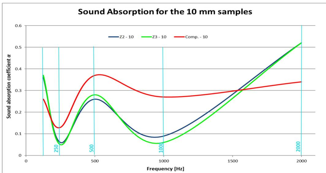
**Figure 6.** Sound absorption of cement composites th. 10 mm.
