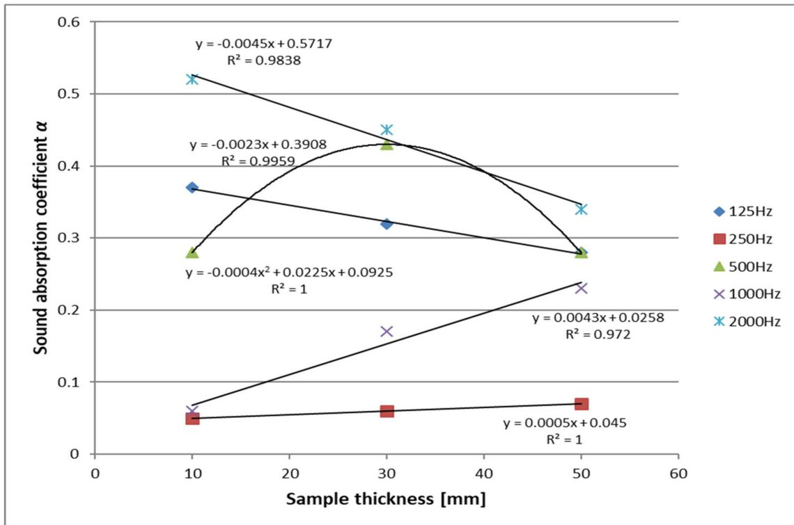
Figure 10. Sound absorption coefficient dependence on the thickness of the sample of mixture Z3 (the trendline is reported for each set of measurements).
