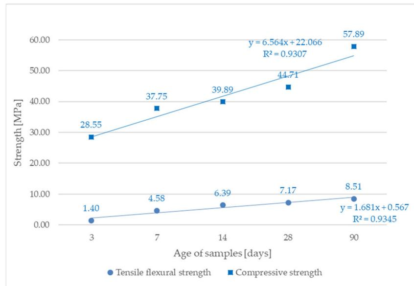
Figure 3. Tensile flexural strength and Compressive strength of comparative mixture.
