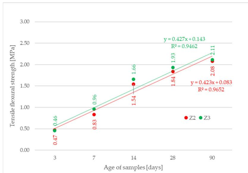
Figure 4. Tensile flexural strength of mixtures Z2 and Z3.
