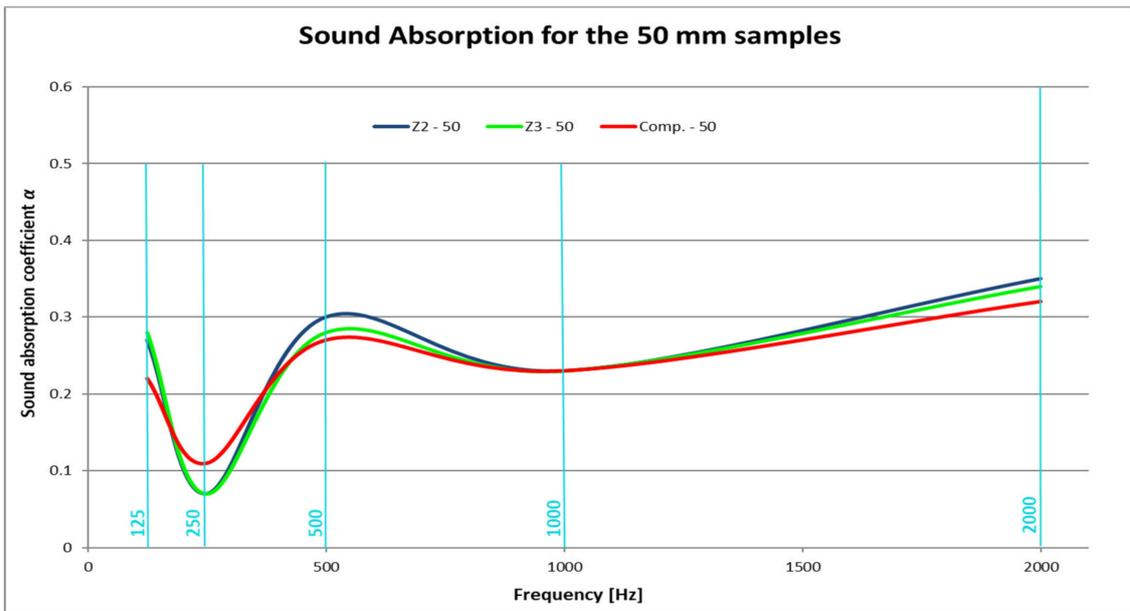
Figure 8. Sound absorption of cement composites (thickness 50 mm).
