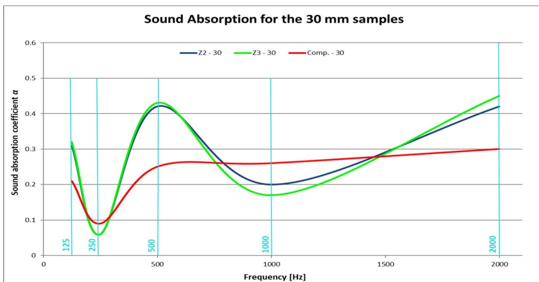
**Figure 7.** Sound absorption of cement composites (thickness 30 mm).
