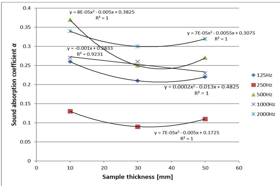
Figure 11. Sound absorption coefficient dependence on the thickness of the sample of comparative mixture (the trendline is reported for each set of measurements).
