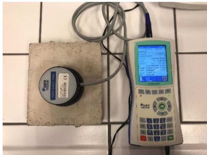
**Figure 1.** Setup used for the measurement of the thermal properties.
