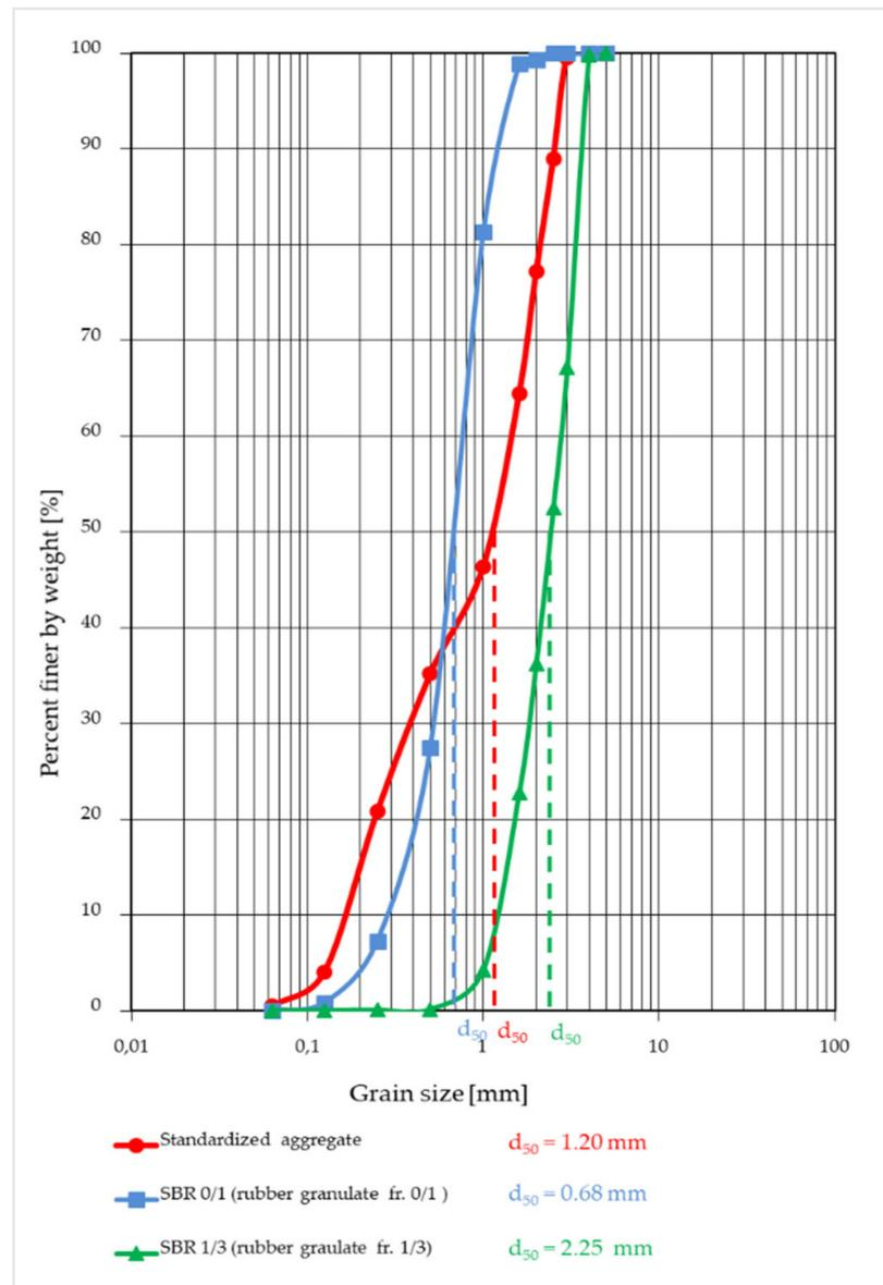
**Figure 2.** Grain size curve of standardized aggregate and rubber granulate fr. 0/1 mm, fr. 1/3 mm.
