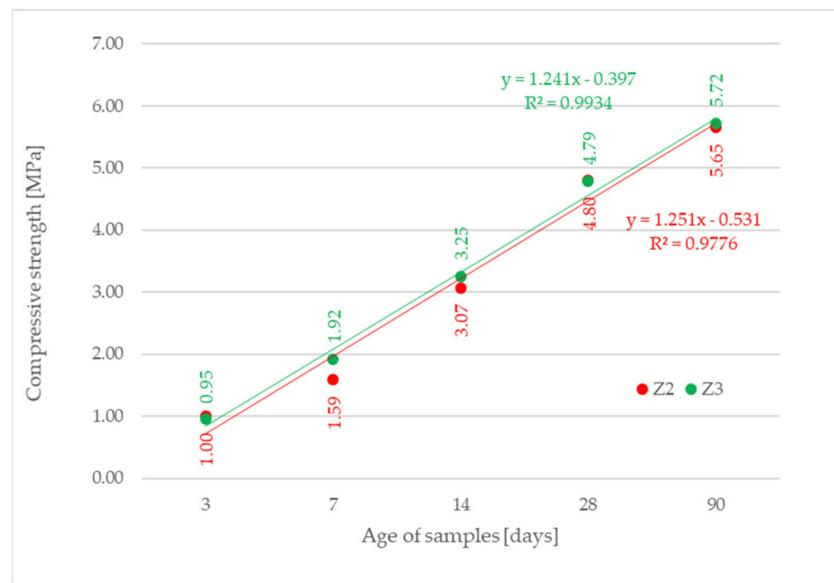
**Figure 5.** Graphical expression of Compressive strength of mixtures Z2 and Z3.
