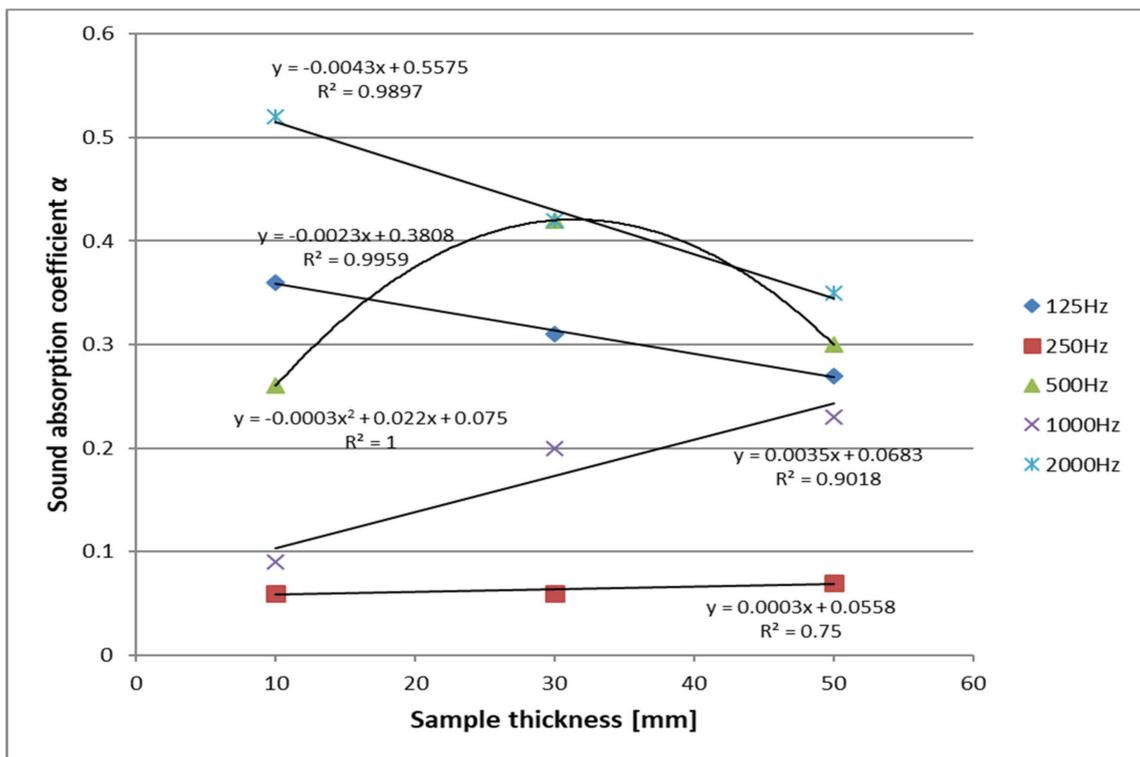
Figure 9. Sound absorption coefficient dependence on the thickness of the sample of mixture Z2 (the trendline is reported for each set of measurements).
