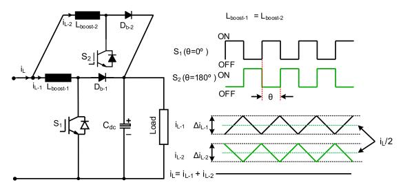
**Figure 4.** Analysis phase shift effects on input ripple current in two units interleaved boost stages. The phase shift between units is considered 180°.
