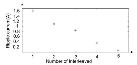
**Figure 6.** Input ripple current on the basis of the number of the interleaved converters with  $f_{sw} = 37.5$  kHz,  $P_0 = 1$  kW, and  $L_{boost} = 1$  mH based on PLECS simulations.
