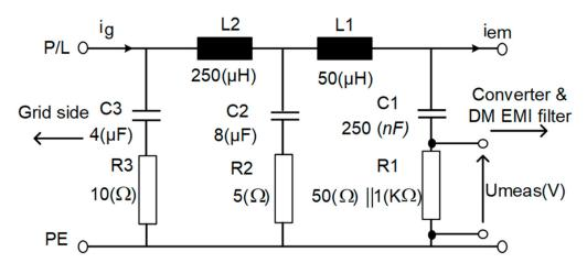
Figure 3. LISN per-phase circuit diagram recommendation by CISPR-16 for 9–500 kHz [9,10].
