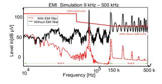
(a) Design EMI filter for band  $B(\theta = 45^{\circ})$
