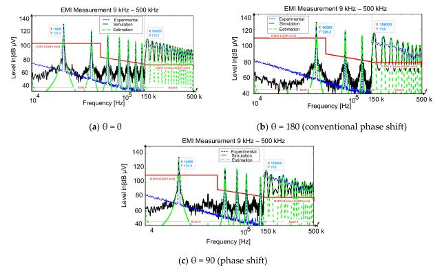
**Figure 15.** EMI results measurement for 2-unit interleaved boost PFC converter, including estimation-based proposed model, simulations, and experiments for different phase shift including (a)  $0^{\circ}$ , (b)  $180^{\circ}$ , and (c)  $90^{\circ}$ . Test system specification is on the basis of results given in Table 5.
