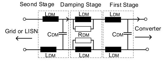
Figure 2. Symmetrical two-stage differential mode (DM) EMI filter configuration.
