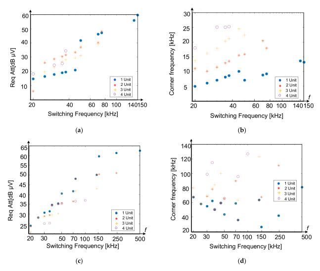
**Figure 5.** Relationship between attenuation requirement and the switching frequency (up to four units interleaved) in (a) Band A. (c) Band-B. The relationship between a two-stage filter corner frequency and switching frequency (up to four units interleaved) in (b) Band A (d) Band B for CCM based on the attenuation requirement (1)–(2). The conventional phase shift is considered 360°/N.
