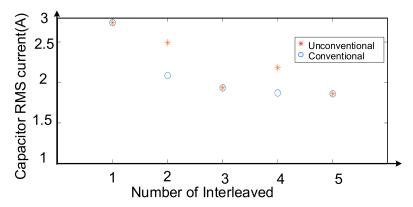
**Figure 9.** Input ripple current of the DC capacitor on the basis of the number of the interleaved converters with  $f_{sw} = 37.5$  kHz,  $P_0 = 1$  kW, and  $L_{boost} = 1$  mH based on PLECS software simulations. The conventional phase shift is considered 360°/N and unconventional is selected based on the (17) and (18).
