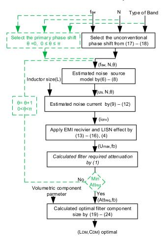
Figure 10. Flow chart of DM EMI filter boxed-volume optimization.
