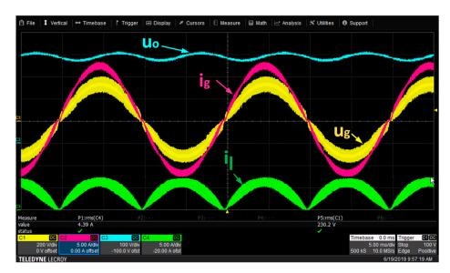
**Figure 14.** Measured waveforms of two units interleaved using parameters ( $f_{sw} = 20 \text{ kHz}$ ) and a phase shift of 180° given in Table 5.
