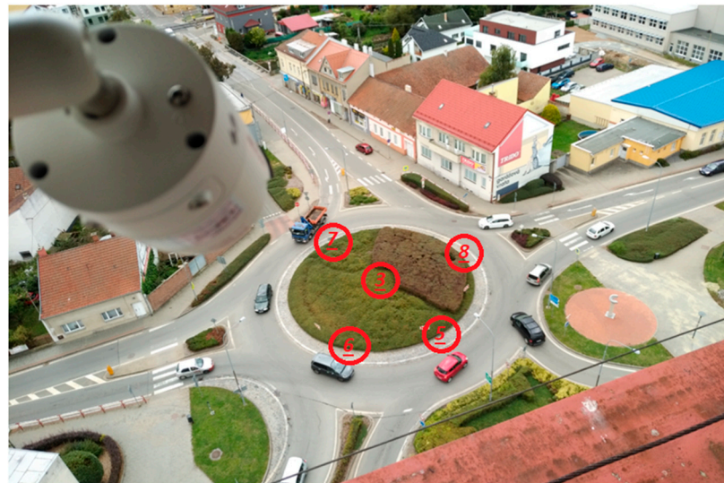
Figure 6. The camera scene over the roundabout, 3, 5, 6, 7, 8 refer to the locations of the microphones.
