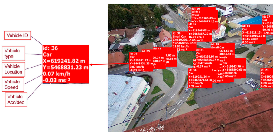
Figure 8. Video pre-processing and vehicle trajectory detection.
