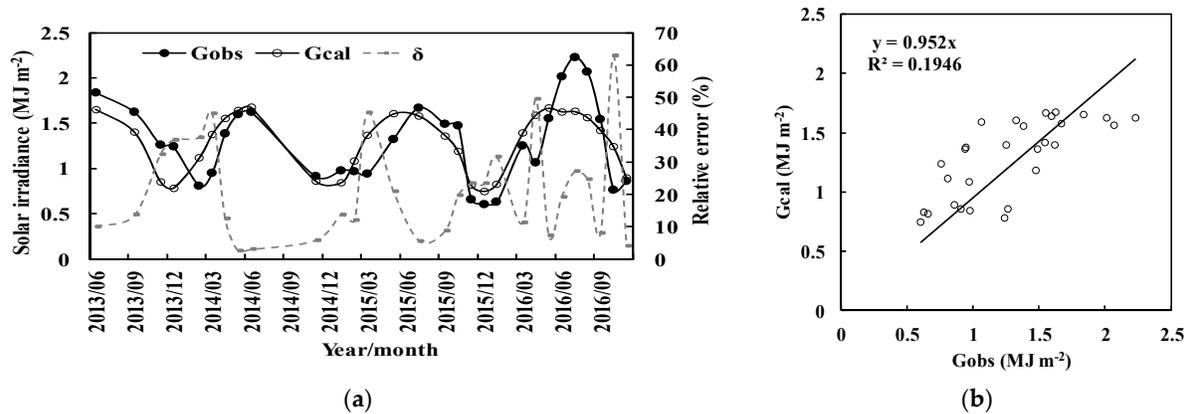
**Figure 2.** (a) Time series of monthly mean calculated and observed global horizontal solar irradiances ( $G_{cal}$  and  $G_{obs}$ ) and their relative errors ( $\delta$ ) for atmospheric conditions with  $S/G \geq 0.8$ . (b) Scatter plot of calculated versus observed solar irradiance ( $G_{cal}$  and  $G_{obs}$ ) for atmospheric conditions with  $S/G \geq 0.8$ . The regression parameters in the legend were obtained for a fit forced through zero.
