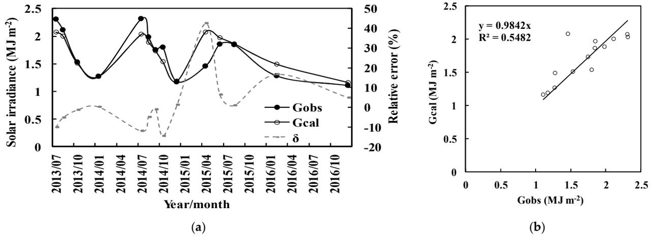
**Figure 1.** (a) Time series of monthly mean global horizontal solar irradiances: calculated solar irradiances ( $G_{cal}$ , from the model Equation (3)), observed solar irradiances ( $G_{obs}$ ), and their relative errors ( $\delta$ ) ( $S/G < 0.80$ ). (b) Scatter plot of calculated versus observed solar irradiance ( $G_{cal}$  vs.  $G_{obs}$ ) ( $S/G < 0.80$ ). The regression parameters in the legend were obtained for a fit forced through zero.
