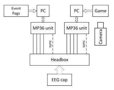
Figure 3. Arrangement of the eight-channeled EEG system.
