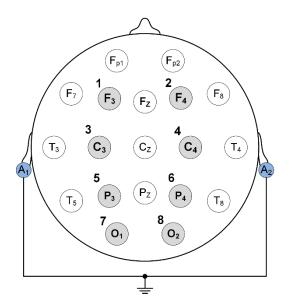
Figure 4. Unipolar electrode configuration for measurement of brain activity.
