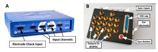
Figure 2. BIOPAC acquisition unit (A) and developed EEG headbox (B).
