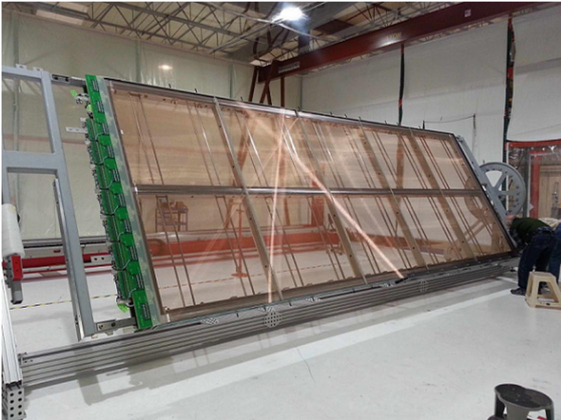
**Figure 25.** A completed APA, with all wire planes in place and on-frame electronics installed. This particular APA is currently installed at the single phase ProtoDUNE (ProtoDUNE-SP) (see Section 2.6), but the design is identical to that of single-phase DUNE (DUNE-SP). Taken from [47].
