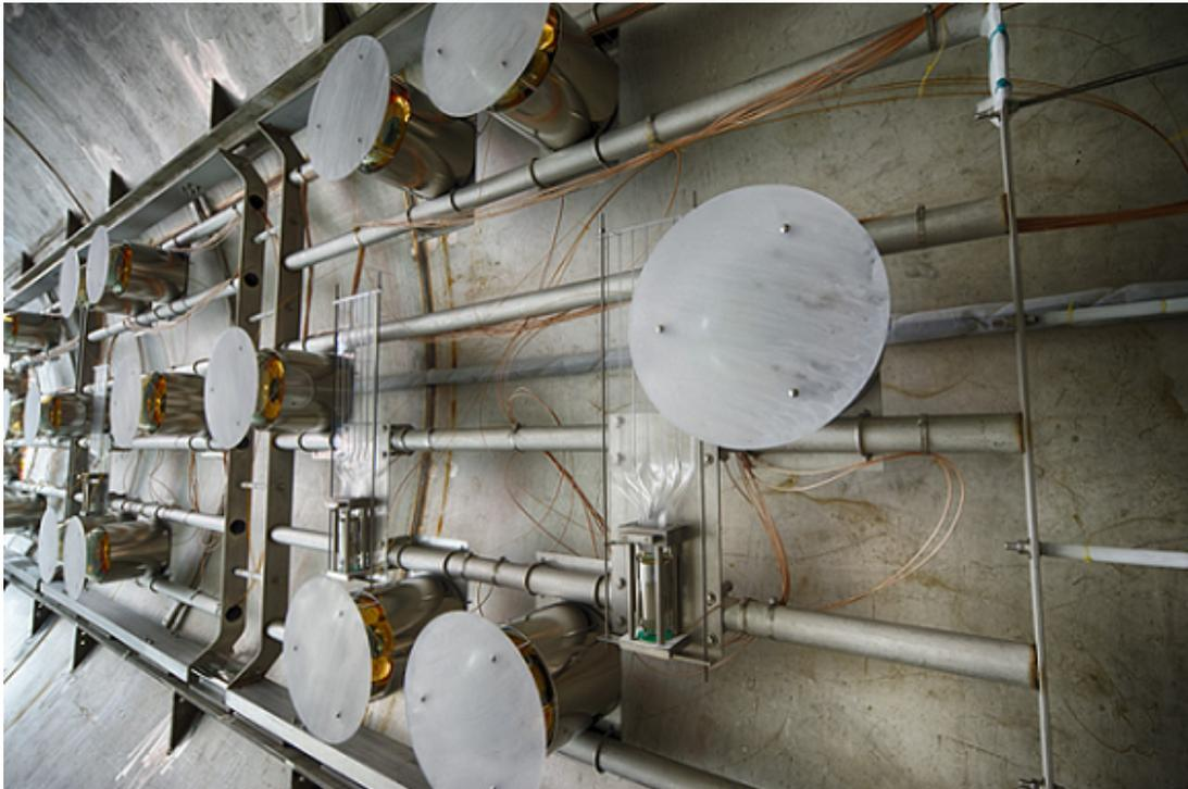
**Figure 12.** The MicroBooNE light collection system mounted on the interior of the cryostat. The two subsystems can be seen: the primary array of 32 8-inch diameter Hamamatsu R5912-02MOD PMTs with attached Tetra-Phenyl Butadiene (TPB)-coated acrylic disks, and the secondary set of 4 (vertically orientated) lightguide paddles. Taken from [12].
