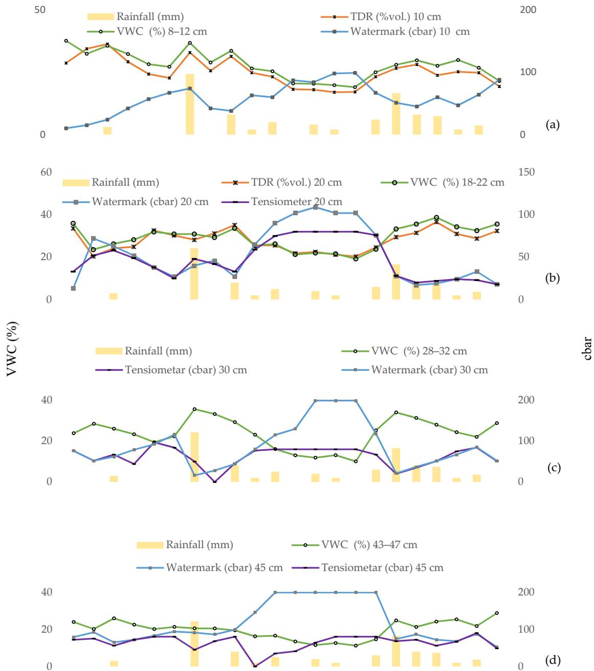
**Figure 5.** Amount of rainfall (mm) and soil water content (Volumetric Water Content (VWC) (%), cbar) at 10 (a), 20 (b), 30 (c) and 45 cm (d).
