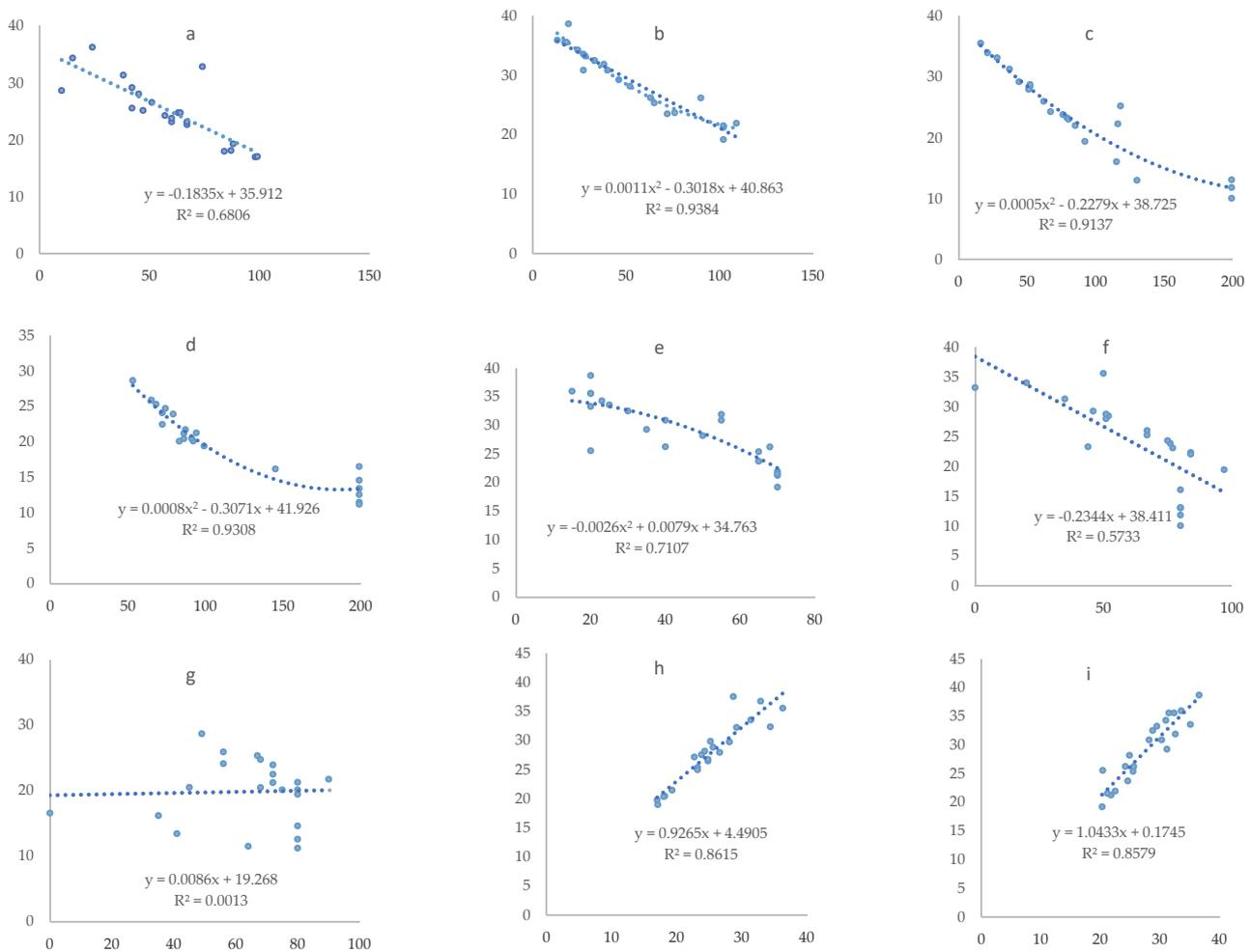
**Figure 6.** (a) Watermark vs. Soil Water Content (SWC) 10 cm, (b) Watermark vs. SWC 20 cm, (c) Watermark vs. SWC 30 cm, (d) Watermark vs. SWC 45 cm, (e) Tensiometer vs. VWC 20 cm, (f) Tensiometer vs. VWC 30 cm, (g) Tensiometer vs. VWC 45 cm, (h) Time Domain Reflectometry (TDR) vs. VWC 10 cm, (i) TDR vs. SWC 20 cm.
