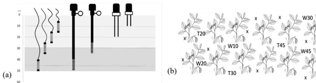
**Figure 4.** The position of tested sensors regarding the monitoring depth (a) and location in the experimental plot (b).
