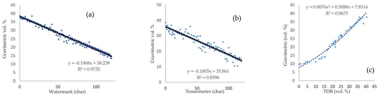
Figure 7. Relationship between sensor readings and laboratory calibrations for Watermark (a), Tensiometer (b) and TDR (c).
