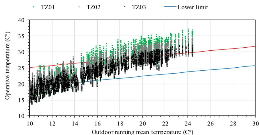
**Figure 13.** Thermal comfort analysis using EN16798-1 for Scenario C.
