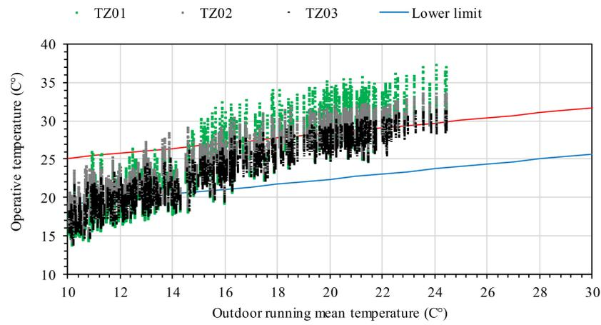
**Figure 14.** Thermal comfort analysis using EN16798-1 for the enhanced solution with BioPCM<sup>®</sup> M<sub>91</sub>/Q<sub>25</sub>\_0.037.
