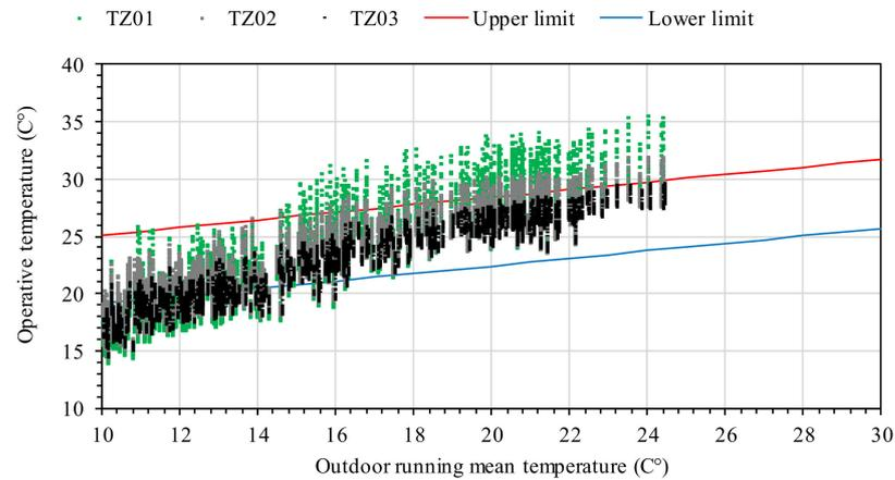
Figure 11. Thermal comfort analysis using EN16798-1 for the reference scenario.
