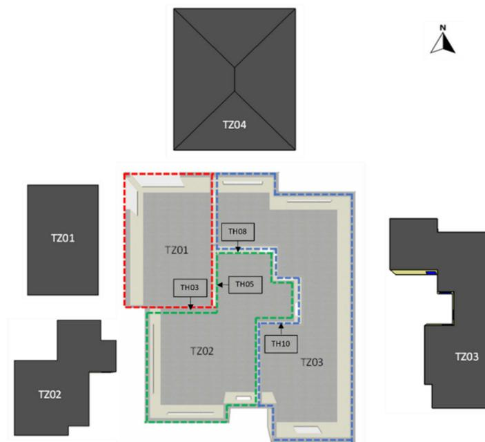
**Figure 7.** Layout of the indoor thermal zones (TZ01, TZ02 and TZ03) and positioning of the monitoring sensors (TH03, TH05, TH08 and TH10).
