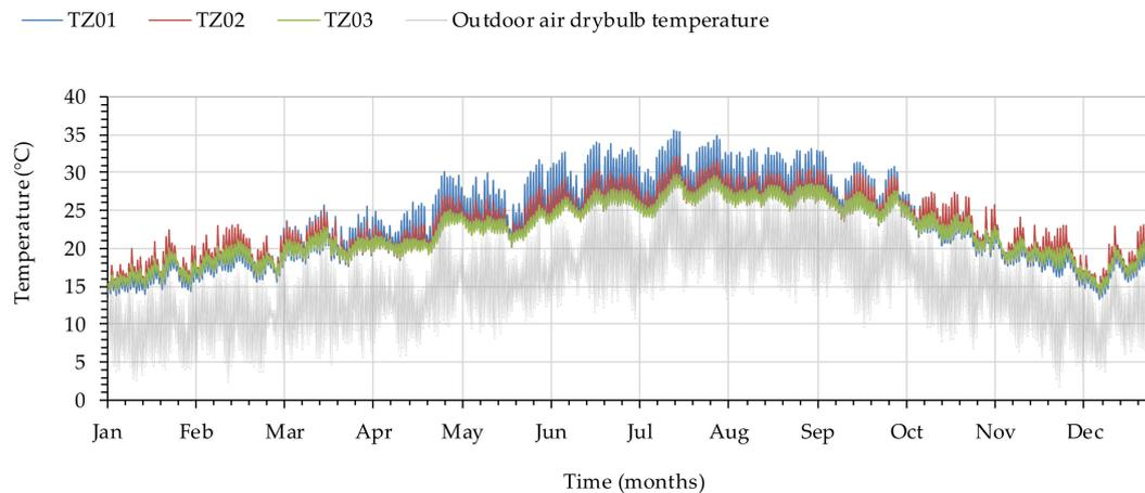
**Figure 10.** Annual temperature of the reference building (indoor and outdoor air dry-bulb temperature).
