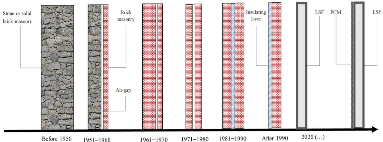
**Figure 3.** Evolution of external wall constructive solutions.
