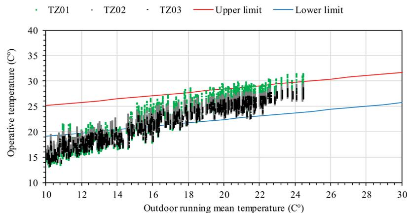
Figure 12. Thermal comfort analysis using EN16798-1 for Scenario B.
