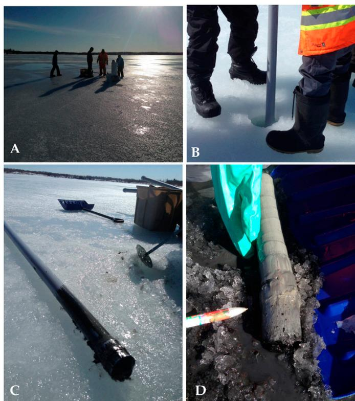
**Figure 2.** Pictures illustrating sample collection during winter, (A) Osisko Lake frozen, (B) driving the polyvinyl chloride (PVC) tube into the hole made in the ice, (C) PVC tube once retrieved containing the sample core, and (D) core sample, with black vase on the first few cm.
