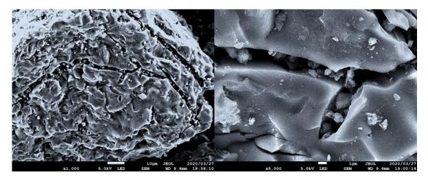
Figure 2. SEM images of the MSC-30 activated carbon.
