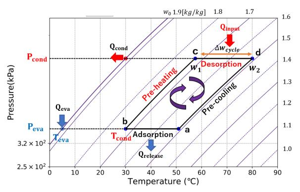
Figure 4. Schematics of the adsorption heat pump cycle.
