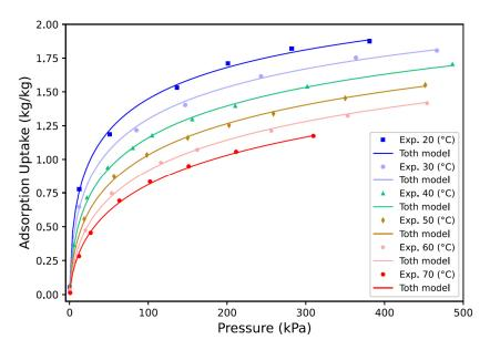
Figure 6. Isotherm fitting results of the Toth model for MSC-30/R1234yf.
