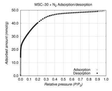
**Figure 1.** Nitrogen adsorption/desorption isotherm ( $T_{iso} = -196$  °C).
