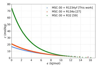
**Figure 8.** Adsorption potential  $\epsilon$  at 20 °C using the parameters of D–A model ( $\alpha = 1/T[K]$ ).
