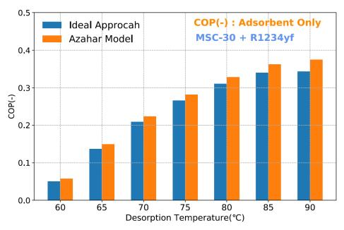
**Figure 12.** COP for heating application of MSC-30/R1234yf, volume correction  $\alpha = 1/T[K]$ .
