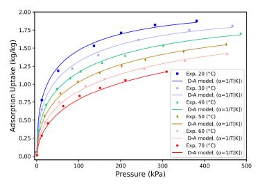
**Figure 7.** Isotherm fitting results of the D–A model ( $\alpha = 1/T[K]$ ) for MSC-30/R1234yf.
