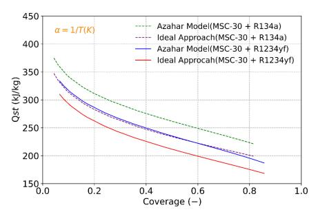
**Figure 9.** Isosteric heat of adsorption using D–A model for MSC-30/R134a and MSC-30/R1234yf pairs at  $30\,^{\circ}$ C.
