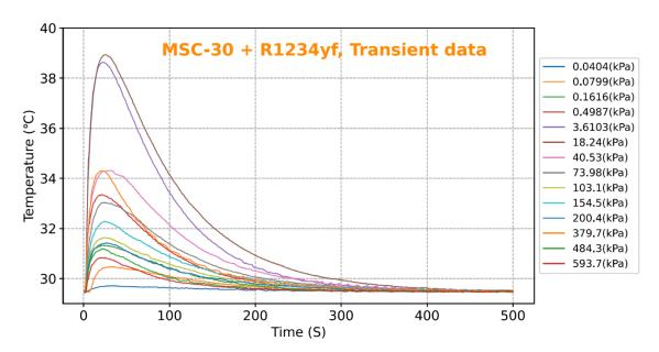
Figure 5. The transient temperature of MSC-30/R1234yf pair at adsorption isotherm (30 °C).
