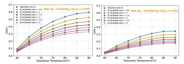
**Figure 11.** (a) Coefficient of performance (COP) for heating application of MSC-30/R134a (Adsorbent mass ratio) with volume correction  $\alpha = 1/T[K]$ , using the ideal approach of isosteric heat of adsorption. (b) COP for heating application of MSC-30/R1234yf (adsorbent mass ratio) with volume correction  $\alpha = 1/T[K]$ , using the ideal approach of isosteric heat of adsorption.
