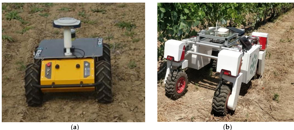
Figure 1. The available agricultural robots that were used in the present analysis, namely (a) Husky and (b) Thorvald robots.
