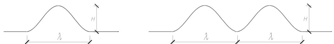
**Figure 7.** Single and multiple bumps characterized by cosine functions.
