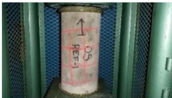
Figure 1. Experimental tests setup of compressive strength test of concrete.
