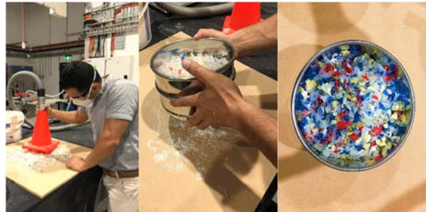
Figure 1. Separating filter fibres from biomedical polymeric waste (BPW) by sieving and vacuuming.
