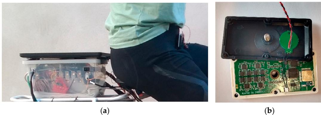
**Figure 2.** (a) Data acquisition system in box with notebook on top and wired connected to the Mcell of the EMG shorts; (b) adapted Mcell for synchronization with the compactDaq and Arduino.
