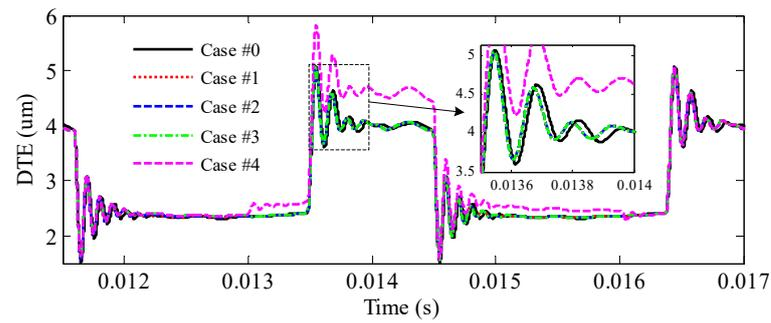
Figure 12. Effects of surface crack propagation on time domain of DTE.
