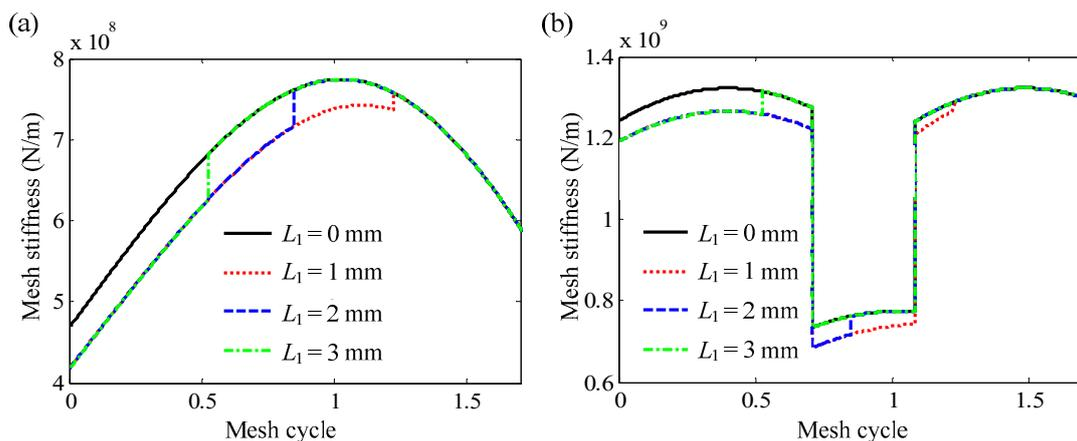
**Figure 5.** Effects of surface crack length on meshing stiffness: (a) single-tooth pair, (b) double-tooth pairs.
