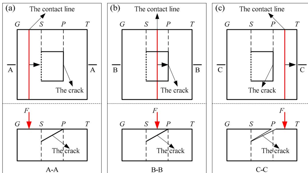
**Figure 3.** Meshing positions of gear tooth with surface crack fault: (a) left of the fault zone, (b) above the fault zone, (c) right of the fault zone.
