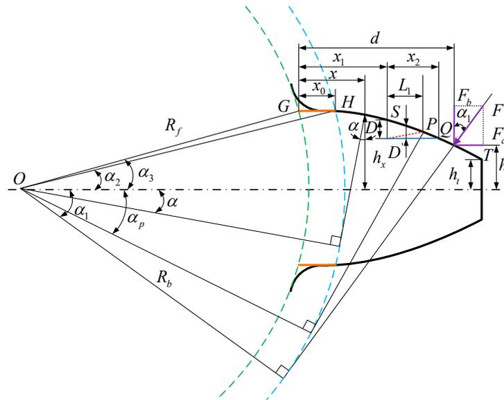
Figure 2. The cantilever beam model of gear with tooth surface crack fault.
