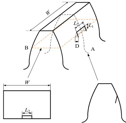
Figure 1. Geometric parameters of tooth surface crack.
