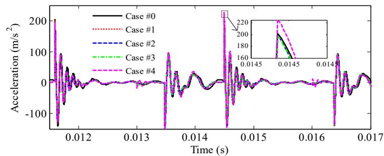
Figure 14. Effects of surface crack propagation on time domain of acceleration response.
