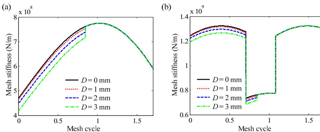
Figure 7. Effects of surface crack depth on meshing stiffness: (a) single-tooth pair, (b) double-tooth pairs.
