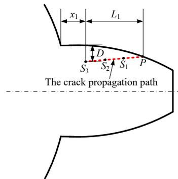
Figure 10. Schematic of surface crack propagation.
