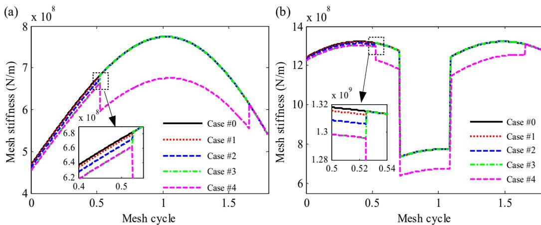
Figure 11. Effects of surface crack propagation on meshing stiffness: (a) single-tooth pair, (b) double-tooth pairs.
