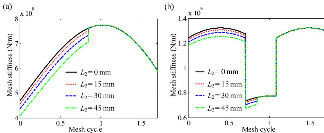
Figure 6. Effects of surface crack width on meshing stiffness: (a) single-tooth pair, (b) double-tooth pairs.
