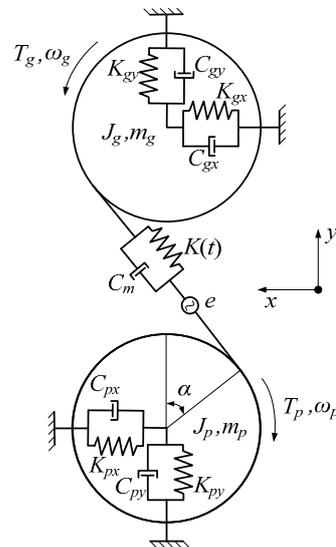
Figure 4. Dynamical model of spur gear system with six DOF.
