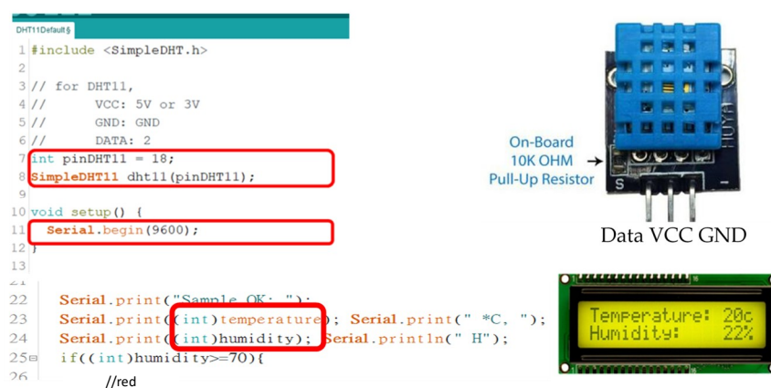
Figure 2. Arduino program-controlled temperature and humidity sensing and LCD synchronous display.
