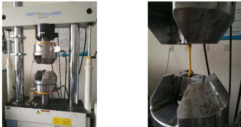
**Figure 3.** The servo-hydraulic machine for tensile test and the specimen.
