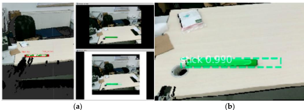
**Figure 10.** The identification result of Mask-RCNN algorithm. (a) Mask-RCNN can recognize the target in real-time. (b) The recognition result of the Mask-RCNN algorithm including Mask region, label, and confidence.
