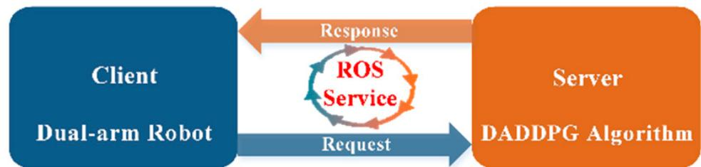
**Figure 7.** The control architecture. The agent of the deep reinforcement learning algorithm is a server and sends a response to the client. The dual-arm robot is a client and requires service from the server.
