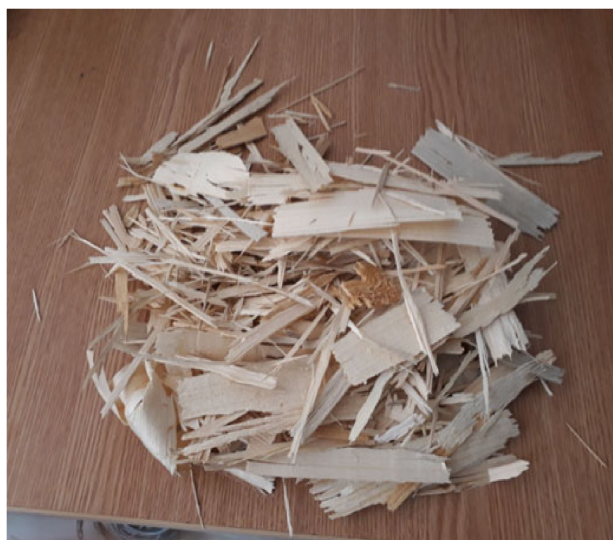
Figure 5. Strand size for OSB boards.
