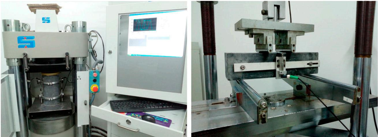
Figure 4. Modulus of elasticity and flexural strength tests.
