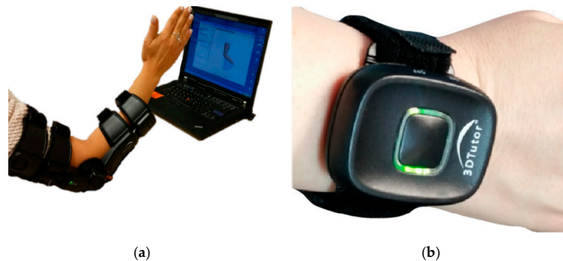
Figure 2. The Meditouch hardware used in this study comprise (a) the ArmTutor device, used for exercising elbow flexion and extension, and (b) the 3-D device, placed on the wrist and used for exercising supination and pronation.
