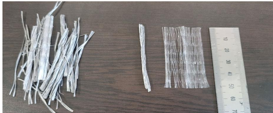
**Figure 1.** Macro-synthetic fiber.**Table 2.** Mix proportions of concrete.
