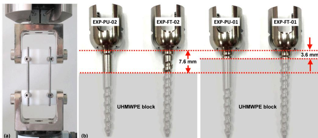
**Figure 1.** (a) American Society for Testing and Materials (ASTM) F1717 standard configuration. (b) Two different setups were evaluated: (i) pedicle screw fully inserted into the test block with an exposed length of 3.6 mm (EXP-FT-01 and EXP-PU-01) and (ii) pedicle screw inserted leaving 7.6 mm of the screw shaft exposed (EXP-FT-02 and EXP-PU-02).
