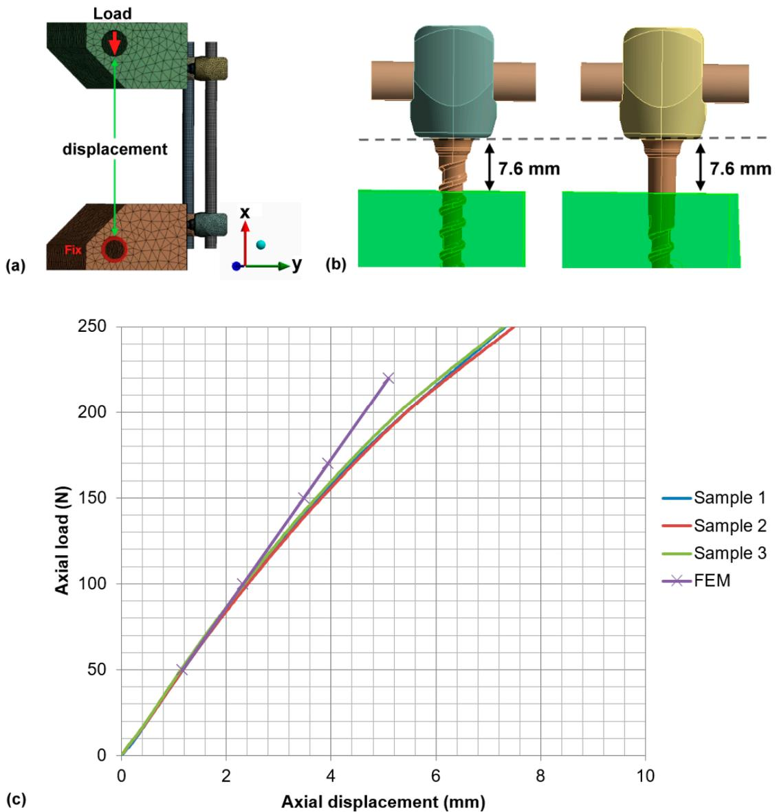
**Figure 2.** (a) Finite element model in accordance with ASTM F1717 standard configuration. (b) Pedicle screw inserted leaving 7.6 mm unsupported length (FEM-FT-02 and FEM-PU-02). (c) The axial displacement and load curve of experimental data of EXP-FT-01 and finite element model FEM-FT-01.
