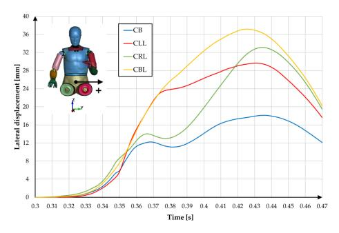
Figure 10. Lateral displacement of dummy H-point.
