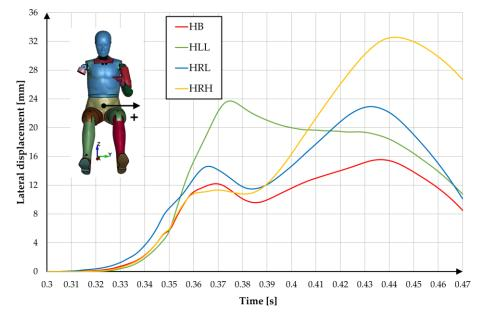
Figure 9. Lateral displacement of dummy H-point.
