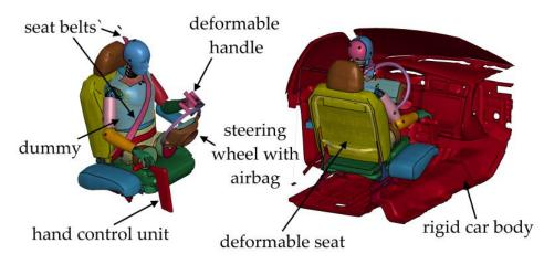
Figure 2. Numerical model used in simulations.
