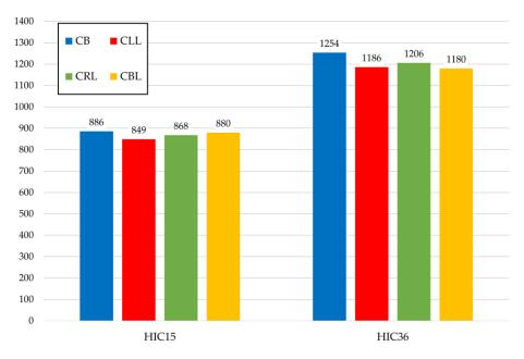
Figure 19. Head Injury Criterion (HIC) comparison.
