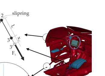
Figure 3. Numerical model of seatbelts.
