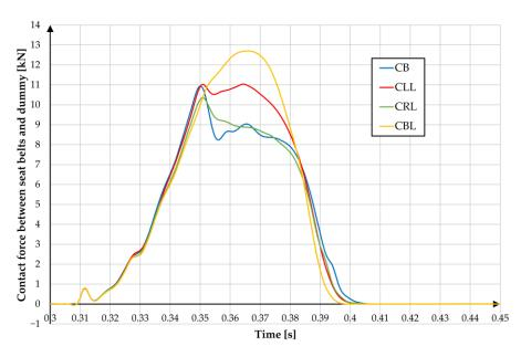
Figure 16. Comparison of contact force between the seat belts and the dummy.
