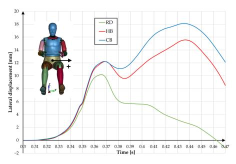
Figure 8. Lateral displacement of dummy H-point.
