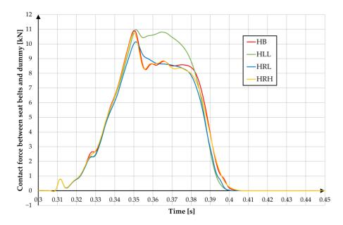
Figure 15. Comparison of contact force between the seat belts and the dummy.
