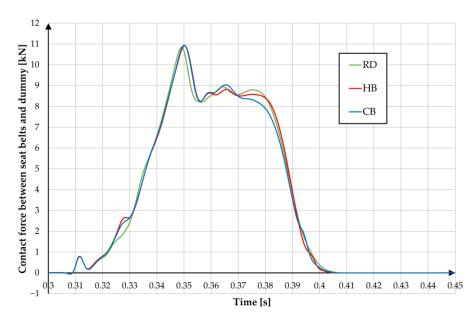
Figure 14. Comparison of contact force between the seat belts and the dummy.
