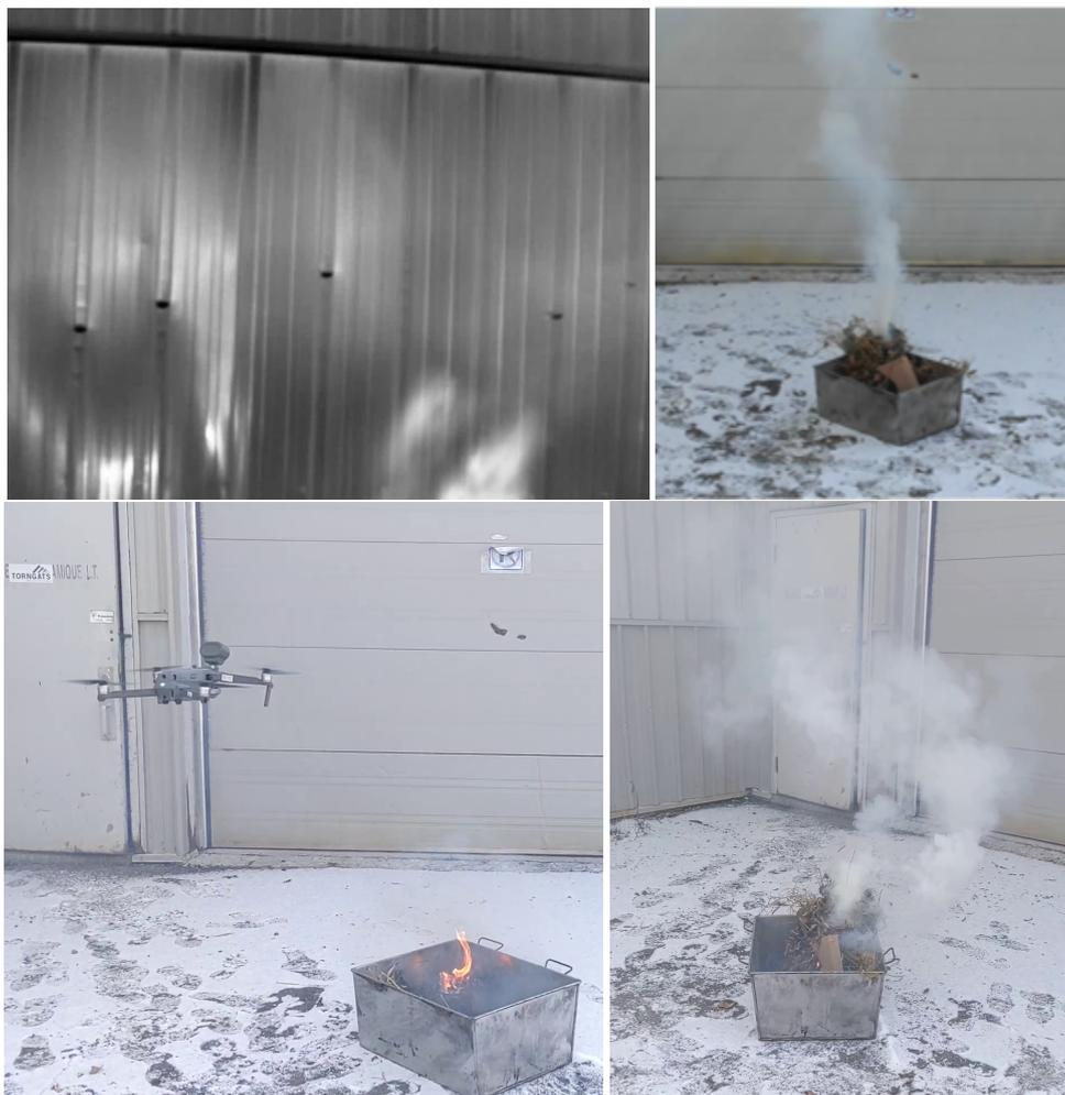
**Figure 5.** Sample photos of the drone-based experiment. The (top left) photo is a thermal image of the gas emission, the (top right) photo is a visible image collected by drone; the (bottom left) is a photo of the drone during the experiment and the (bottom right) is another photo sample of collected imagery data by drone.
