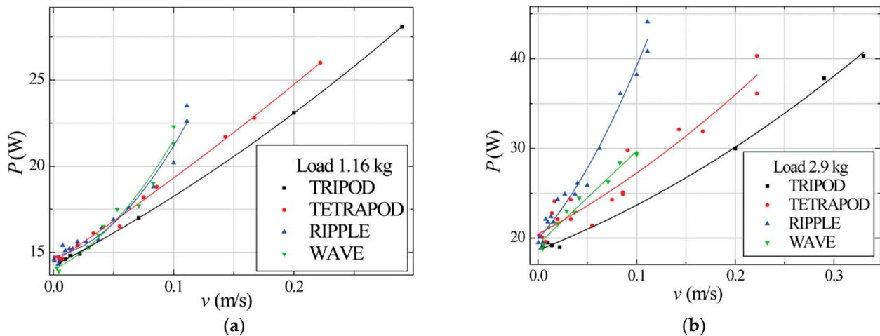
**Figure 4.** Average power dependence on robot speed and gaits with different robot loads: (a) 1.16 kg load, (b) 2.9 kg load. Each dot represents a separate experiment with a certain configuration. Lines show polynomial approximation. No gait switching was used.
