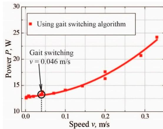
**Figure 7.** Influence of gait switching on energy consumption. Speed for switching from wave gait to tripod gait is equal to 0.046 m/s.
