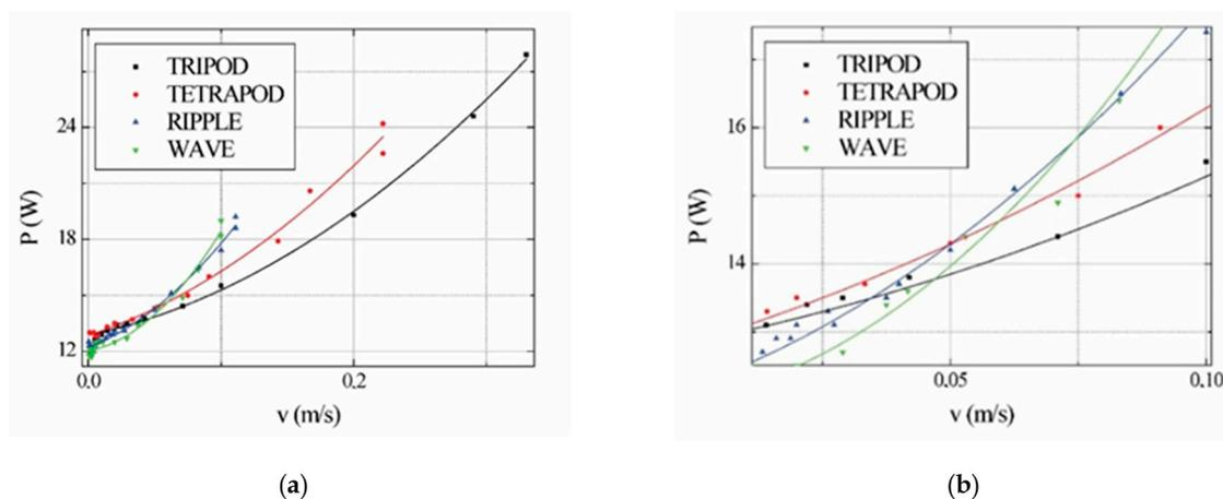
**Figure 3.** Average power dependence on robot speed and gaits: (a) normal view, (b) enlarged view. Experiments were carried out without additional load on the robot. Each dot represents a separate experiment with a certain configuration. Lines show polynomial approximation. No gait type switching was used.
