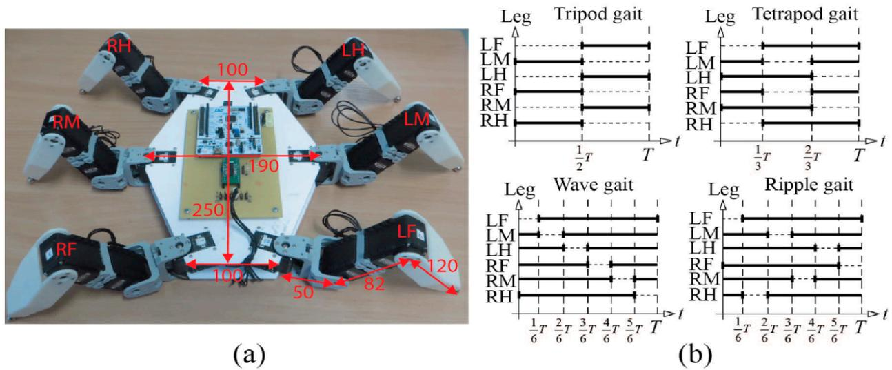
**Figure 1.** Hexapod robot model HexaV4 (a) and gait used in experiments time diagrams (black lines represent leg’s support phase, dashed gap—transfer phase) (b). Leg abbreviations: LF—left front; LM—left middle; LH—left hind; RF—right front; RM—right middle; RH—right hind; T—gait period. All dimensions are in millimeters.
