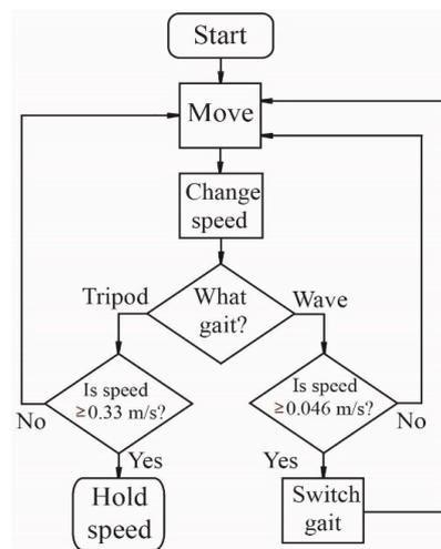
**Figure 2.** Algorithm for switching between wave and tripod gaits. Wave gait is used when the movement speed is lower than 0.046 m/s; tripod gait is used when the movement speed is higher than 0.046 m/s until the speed reaches a maximum value of 0.33 m/s.
