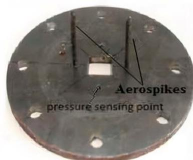
Figure 12. Control plates with aerospike [21].
