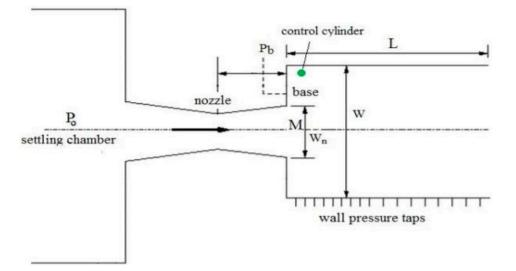
Figure 11. Experimental setup [20].
