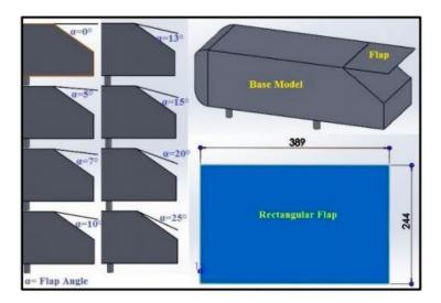
**Figure 14.** Ahmed body with 35° slant angle detailed view with rectangular flap (dimensions in mm) [38].
