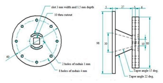
Figure 7. Square nozzle and grooved control plate [7].
