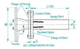
Figure 13. Square nozzle with threaded spikes control plate [23].
