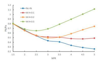
**Figure 9.** Base pressure changes when NPR is increased from 1.5 to 5, and the aspect ratio is changed from 3:1 to 3:3 [18].
