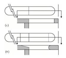
Figure 8. Ventilation slots details (A) with square-edged (B) tapered [10].
