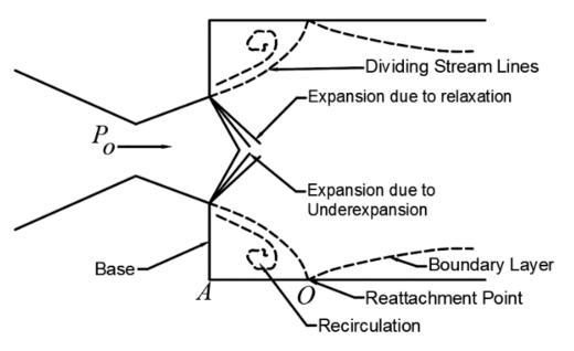
Figure 3. Schematic diagram of the under-expanded flow field.
