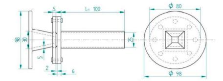
Figure 10. Dimensions of nozzle and duct [19].
