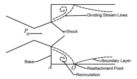
Figure 2. Schematic diagram of over-expanded flow field.
