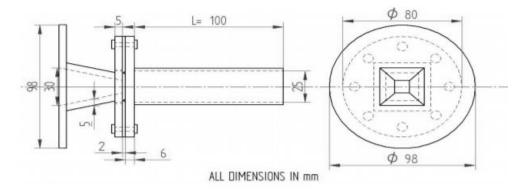
Figure 6. Dimensions of the nozzle and the duct [6].
