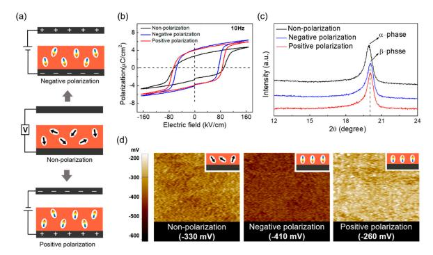
**Figure 3.** (a) Schematic diagrams of three different polarizations: negative polarization, non-polarization and positive polarization. (b) P-E curves of PVDF-TrFE after three different polarization processes. (c) X-ray diffraction (XRD) analysis of PVDF-TrFE, depending on the polarization direction. (d) Kelvin probe force microscopy (KPFM) images of the PVDF-TrFE surface for different polarizations scanned over an area of  $25 \,\mu m^2$ .
