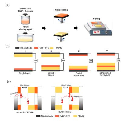
**Figure 1.** (a) Schematic fabrication process by the solution spin coating method. (b) Schematics showing four different contact friction pairs, consisting of polydimethylsiloxane (PDMS) and poly(vinylidene fluoride-co-trifluoroethylene) (PVDF-TrFE) layers. (c) Schematic diagram showing the charge trapping mechanism for two different buried layers: buried PVDF-TrFE (left) and buried PDMS (right).
