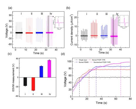
**Figure 2.** (a) Output voltage and (b) current density measured from each triboelectric generator (TEG). The inset is the detailed response of the voltage and current density. (c) Electrostatic voltmeter (ESVM) measurement of four TEGs after several contact–separation motions. (d) The saturated output voltage of four TEGs used in this study.
