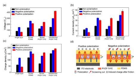
**Figure 4.** (a) Output voltage, (b) current density and (c) charge density measured from four different friction pairs, shown in Figure 1b, after non-, negative and positive polarization of the PVDF-TrFE layer. (d) Suppression of the triboelectrically induced positive surface charge screening effect by the positively polarized PVDF-TrFE layer (left) and screening of the triboelectrically induced positive surface charges by the negatively polarized PVDF-TrFE layer (right).
