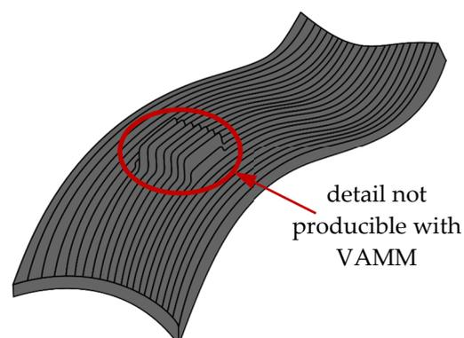
**Figure 5.** Schematic of a CFRP-part including a detail not producible with VAMM in the central part.
