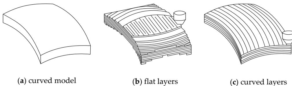
**Figure 16.** Comparison of flat and curved layer manufacturing: (a) curved part to be manufactured (b) part sliced with classical flat layers (c) part sliced with curved layers (based on the work in [92]).
