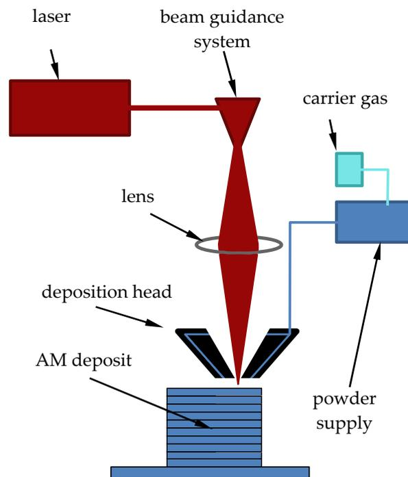
**Figure 10.** Schematic representation of directed energy deposition (based on the work in [29]).
