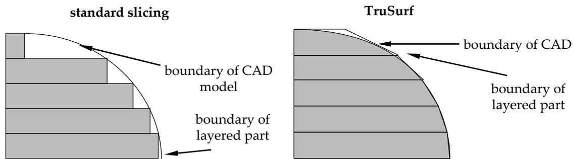
**Figure 15.** Comparison of the staircase effect between standard slicing and the TruSurf algorithm (based on the work in [52]).
