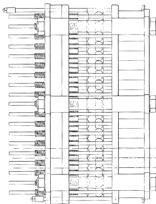
**Figure 2.** Schematic drawing of the first multipoint mould (based on the work in [3]).
