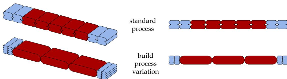
**Figure 14.** Layer configuration in standard fused filament fabrication and the process variation approach (based on the work in [77]).
