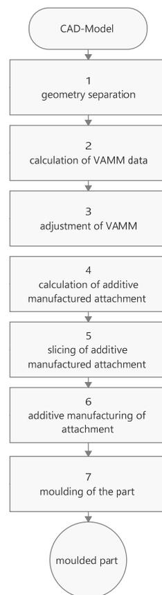
**Figure 7.** Process flow chart for enhanced vacuum assisted multipoint moulding with additive attachments.
