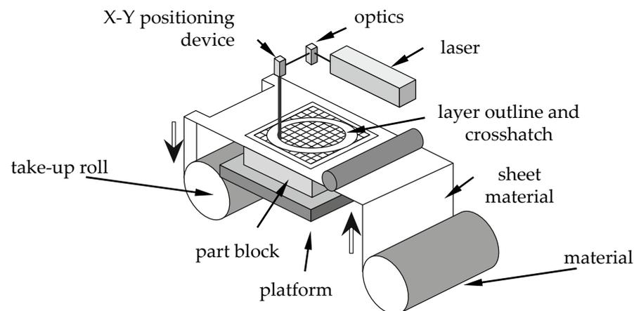
**Figure 13.** Schematic representation of laminated layer manufacturing (based on [50]).
