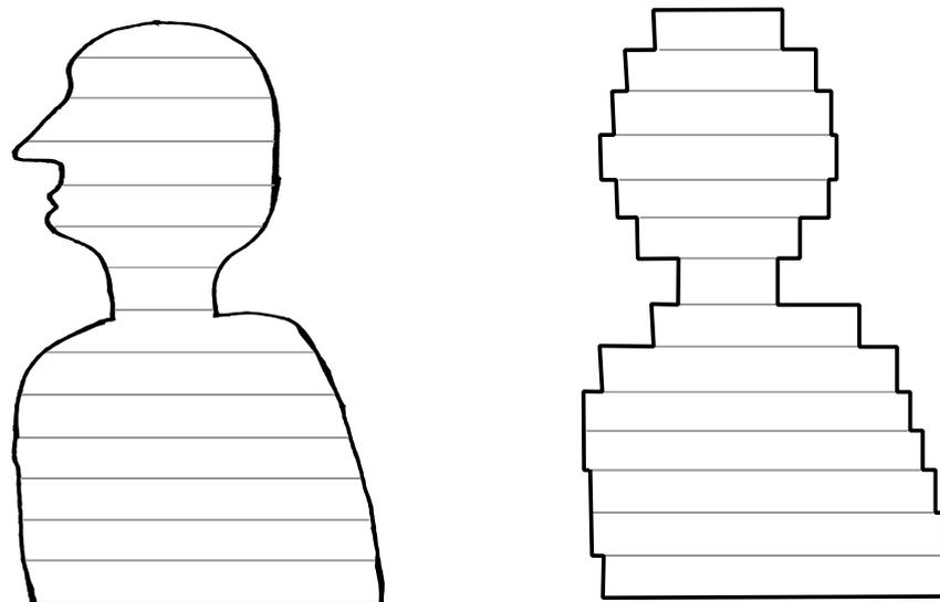
**Figure 8.** Slicing scheme for flat layers in additive manufacturing. Model with marked layers (**left**) and derived layer model (**right**).
