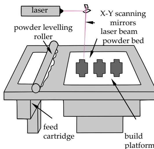
**Figure 9.** Schematic representation of laser powder bed fusion (based on the work in [30]).
