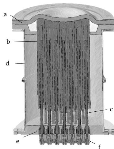
**Figure 3.** Principle of vacuum-assisted multipoint moulding (VAMM), shown in a smaller test setup. The setup from top to bottom: (a) interpolation layer, (b) pin array, (c) threaded rods, (d) vacuum container, (e) base plate and (f) actuator couplings [23].
