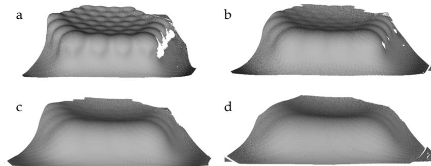
**Figure 4.** 3D scans of bowl shape created with a silicon rubber interpolation layer (40 Shore-A) with varying thickness ((a) 5 mm, (b) 10 mm, (c) 15 mm and (d) 20 mm) at a vacuum of 100 hPa [23].
