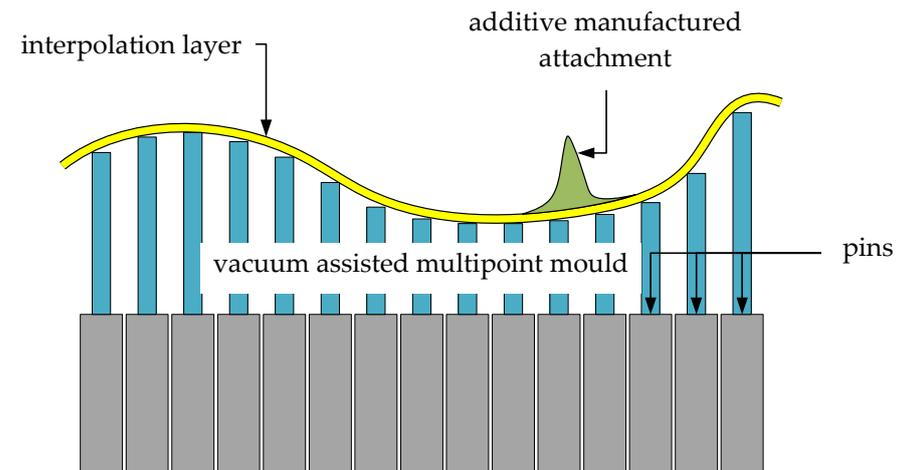
**Figure 6.** Enhanced vacuum-assisted multipoint moulding with additive attachments, consisting of the vacuum-assisted multipoint mould with pins and interpolation layer and the additive manufactured attachment mounted on top of the interpolation layer.
