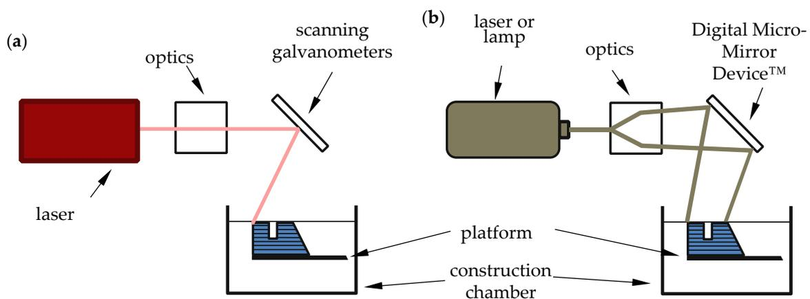
**Figure 12.** Schematic representation of stereolithographic processes: (a) vector scan SLA, (b) mask projection SLA (based on [30]).
