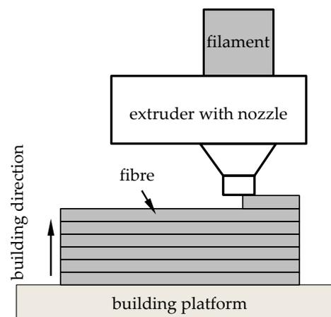
**Figure 11.** Schematic representation of fused filament fabrication (based on the work in [37]).
