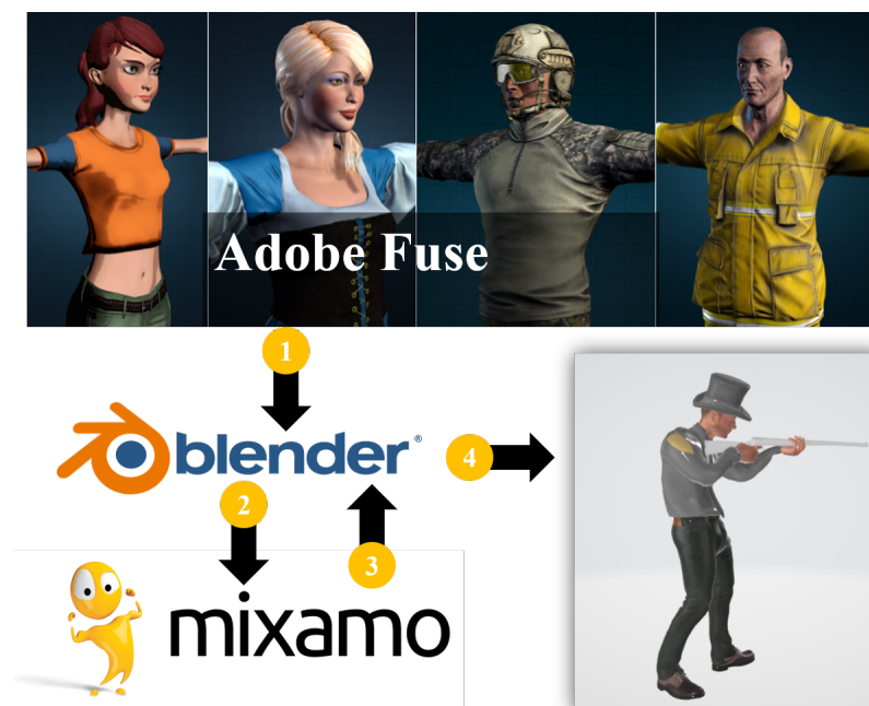
Figure 7. The process of constructing animated character: (1) create a character with a T-pose, (2) customize the model, (3) generate animations, and (4) combine animations and export to GLB format.
