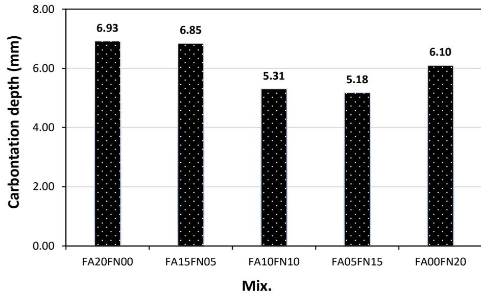
Figure 7. Accelerated carbonation depth.
