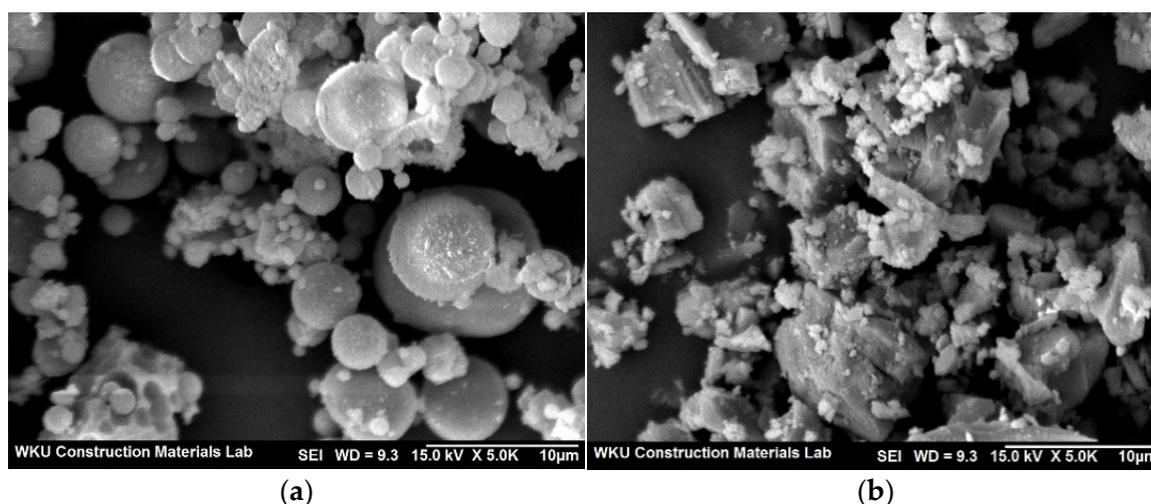
Figure 2. SEM images of sample: (a) fly ash, (b) ferronickel-slag powder.
