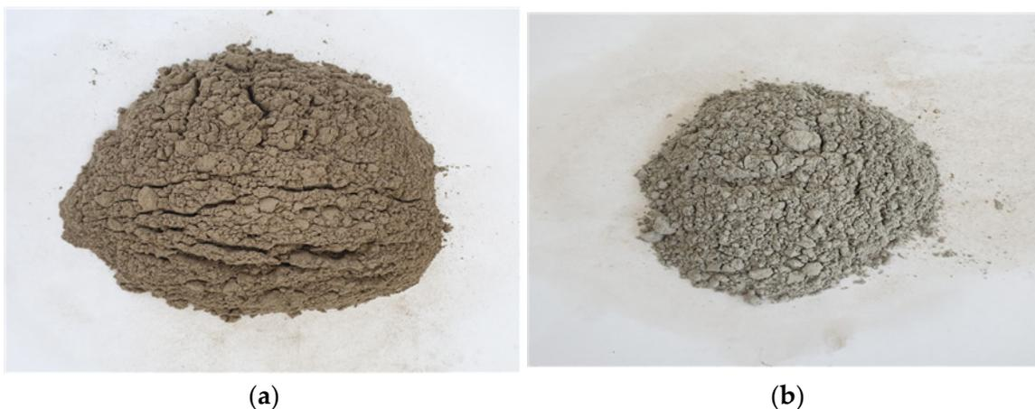
**Figure 1.** Fly ash and ferronickel-slag powder sample: (a) fly ash, (b) ferronickel-slag powder.
