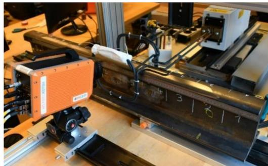
**Figure 1.** The setup for measuring railway rails in the laboratory.
