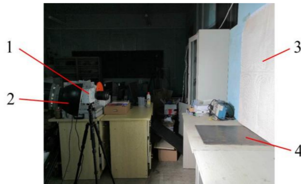
Figure 2. Ear drop test. (1) High-speed camera; (2) light supplement lamp; (3) height marker; (4) steel plate.
