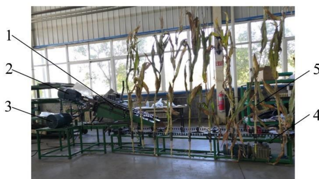
Figure 8. Test device. (1) Low-damage snapping mechanism; (2) rotational speed regulating motor of stalk roller; (3) speed regulating motor of feeding chain; (4) plant feeding mechanism; (5) corn plants.
